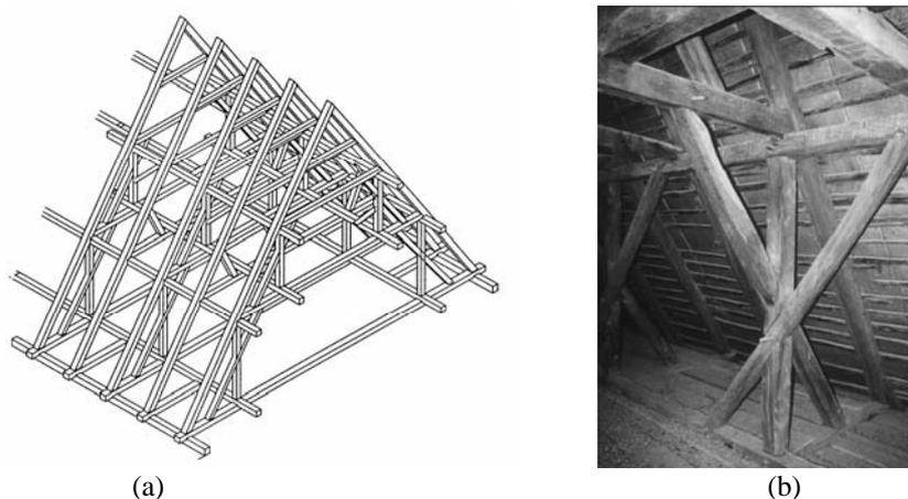
Figure 2 : Gothic roof structure on common rafters and tie-beams with collar beams
