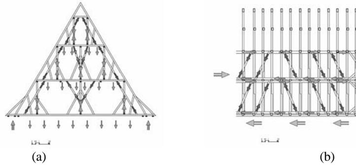
Figure 4 : Gothic roof structure on common rafters and tie-beams with collar beams, (a) Main transverse frame (b) Longitudinal frame
