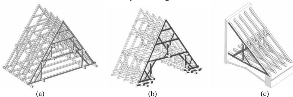
Figure 1 : Gothic roof structures (a) on common rafters and tie-beams with collar beams, (b) on trestles, (c) on common rafters and plates
