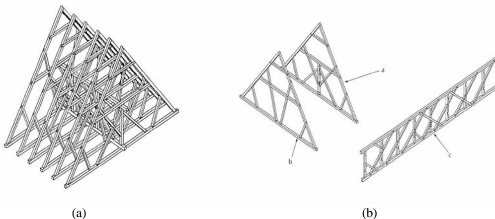
Figure 3 : Frames in Gothic roof structures on common rafters and tie-beams with collar beams, (a) unit, (b) frames
