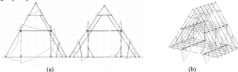
Figure 8 : Efforts in the roof elements of the southern aisle of the Lutheran church in Sibiu (a) frames (b) 3D
