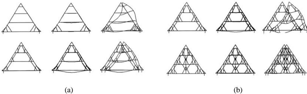
Figure 5 : Deformations in the Gothic roof structures on common rafters and tie-beams with collar beams, at (a) symmetrical, (b) non-symmetrical actions
