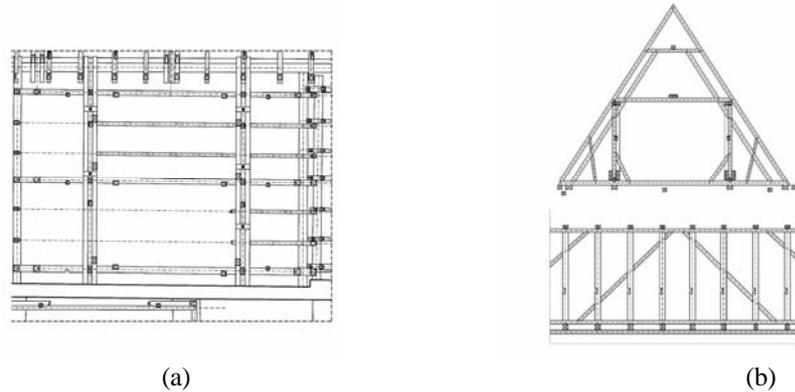
Figure 7 : The roof of the southern aisle of the Lutheran church in Sibiu (a) plan, (b) frames
