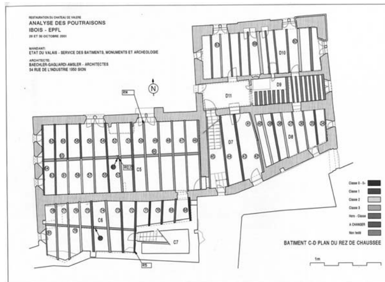
Figure 10 : Monitoring displaying the Sylvatest-Duo results with a specific colour for each wooden beam according to the standards resistance classes.
