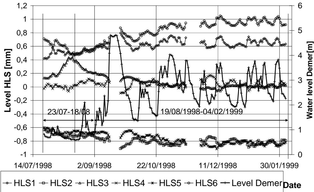
Figure 3 : Water level of the 6 HLS-measuring devices and the river Demer
