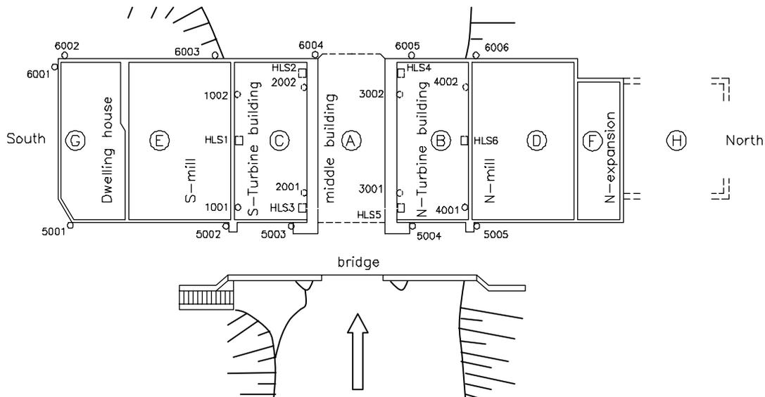
Figure 2 : Hertogen's models (E: Duke's Mill), ground plan, HLS-network and points for geodetic survey.
