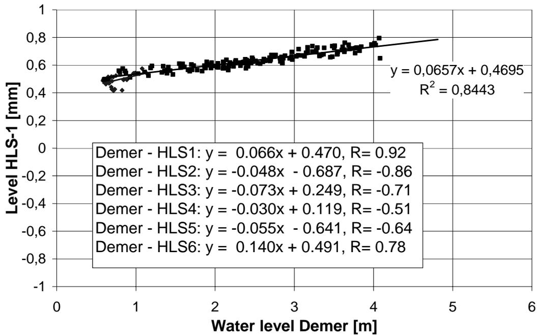
Figure 5 : Water level Demer versus level of HLS-measuring device
