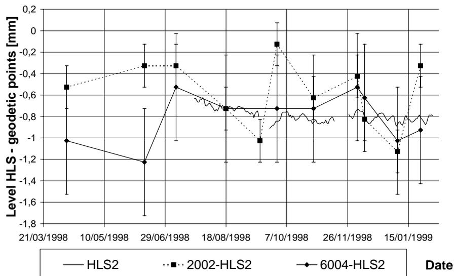
Figure 6 : Example of the geodetic survey at points 2002 and 6004 - comparison with HLS-2.
