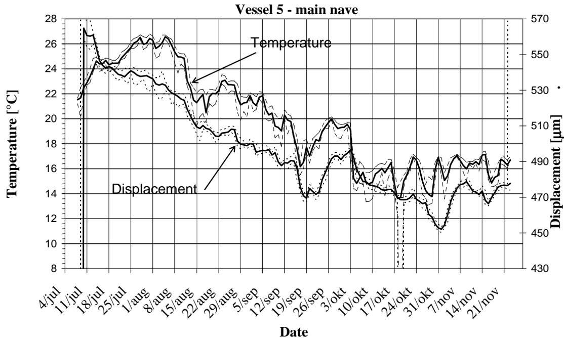
Figure 8 : Temperature and displacement as function of time – vessel 5 – main nave
