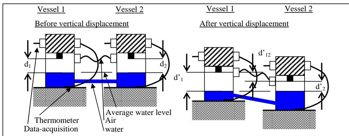
Figure 1 : Hydrostatic levelling system – measuring principle
