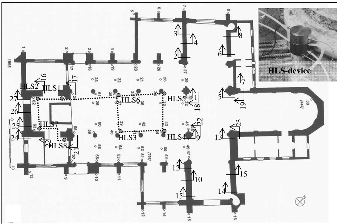
Figure 7 : Position of topographic levelling points, Hydrostatic levelling System and vertical profiles
