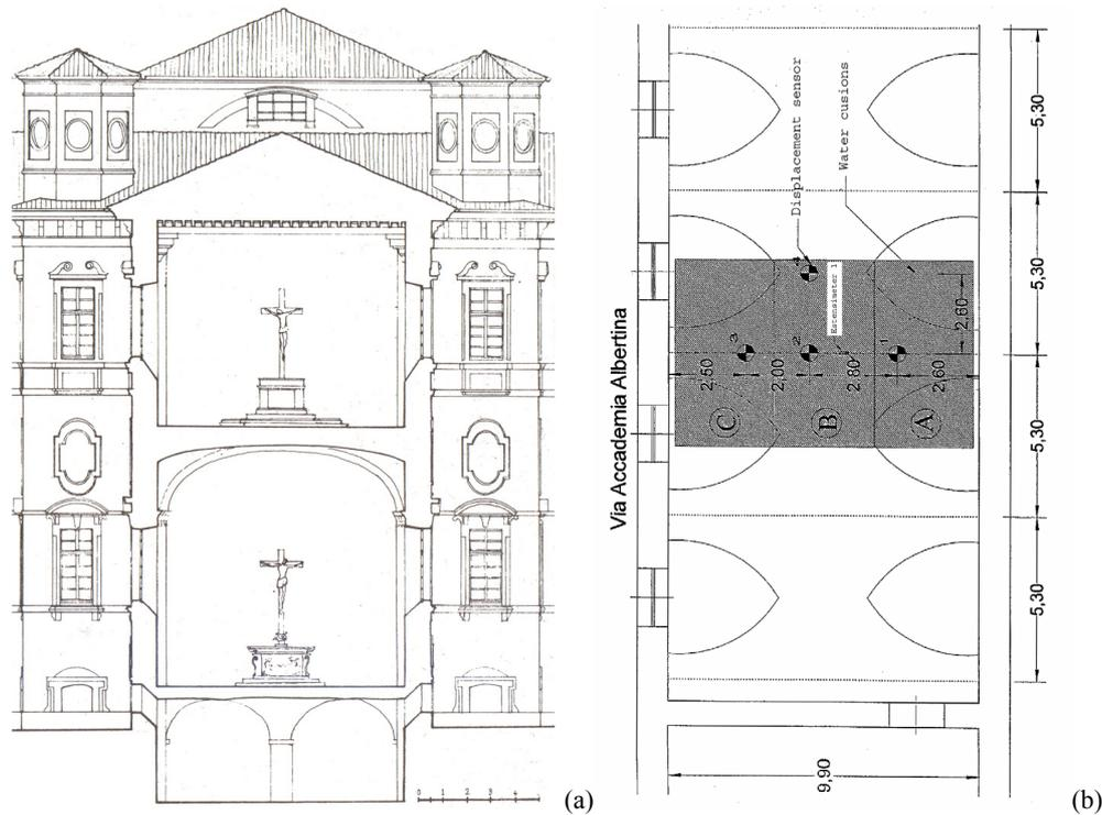
Figure 2 : (a) Section of the building; (b) scheme of the barrel vault with indication of the water cushions (A, B and C) and positions of the measurement points.
