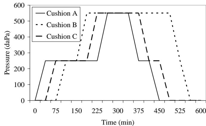
Figure 3 : diagram of the loading and unloading procedure.
