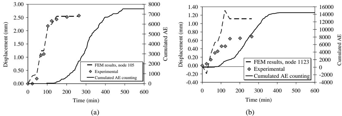
Figure 11 : comparison between cumulated AE counting (right y-axis) and the experimental or FEM vertical displacements (left y-axis).
