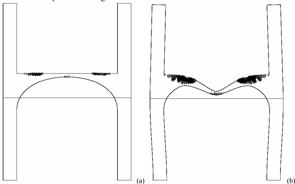
Figure 9 : (a) Crack pattern at the maximum experimental load; (b) and at the ultimate load.
