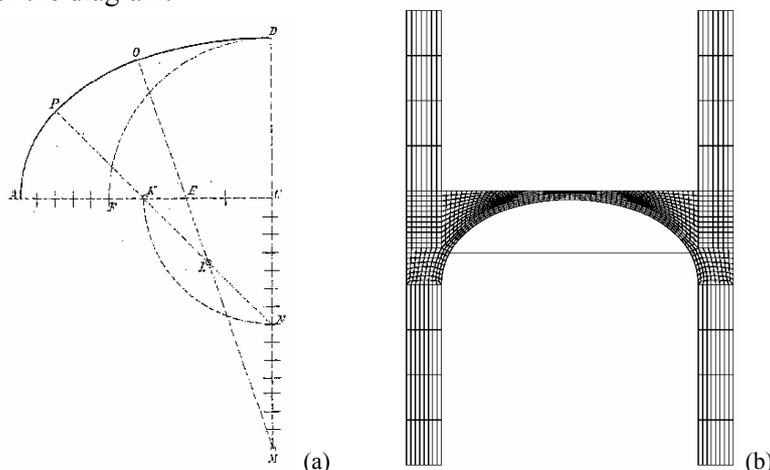
Figure 6 : (a) Approximate construction of the polycyclic vault line; (b) mesh of the FEM model.
