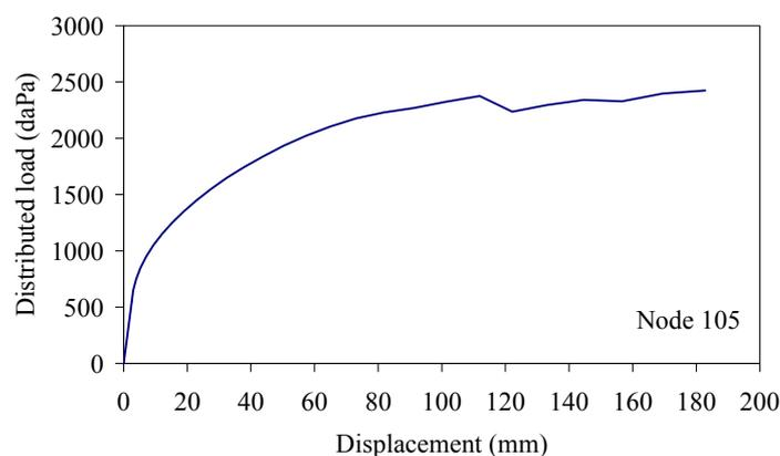
Figure 10 : Complete load vs. displacement curve (at node 105).
