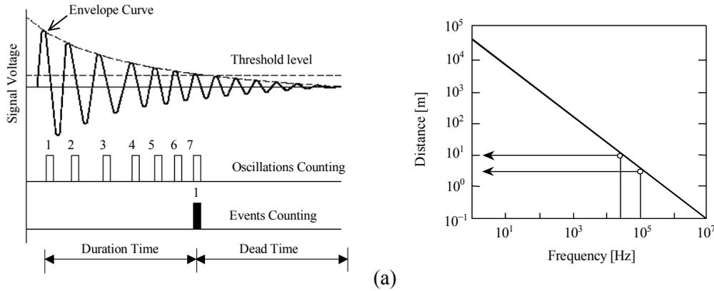
Figure 4 : (a) Signal identified by the transducer and counting methods in AE technique; (b) acoustic emission relationship between signal detection distance and signal frequency.
