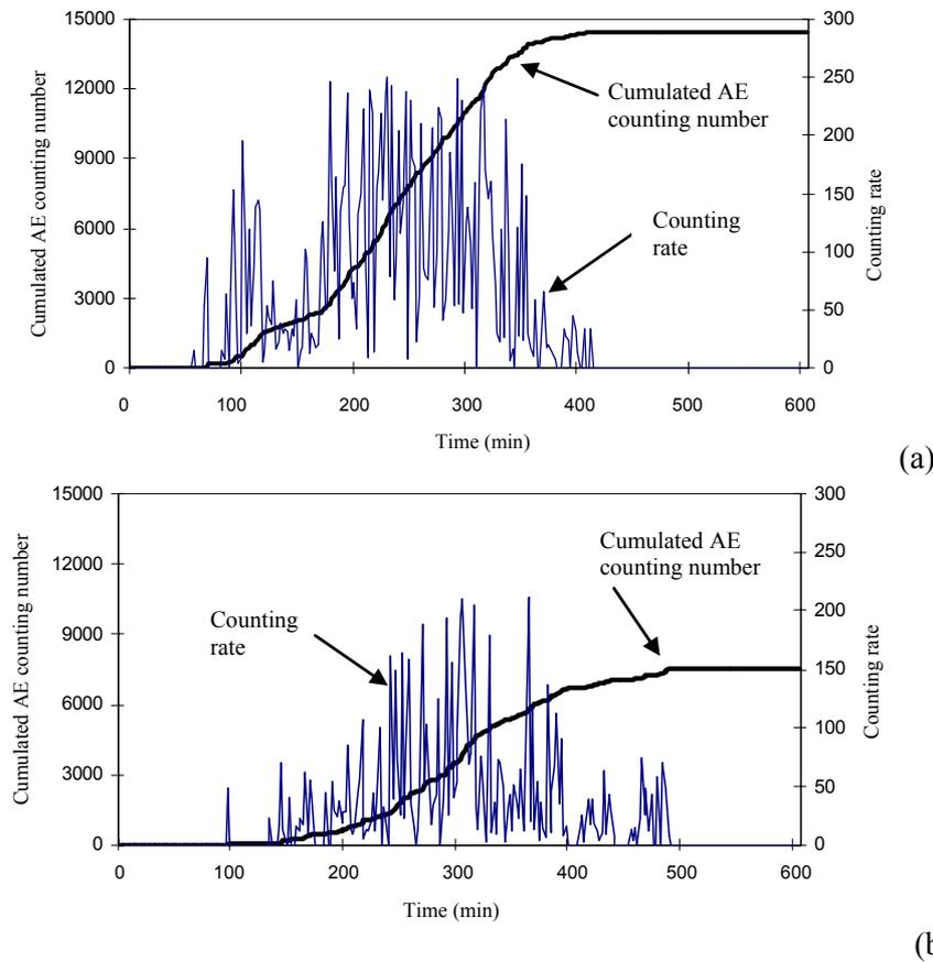
Figure 5 : (a) AE signal of the sensor in position 1; (b) and close to the vault key, sensor in position 2.
