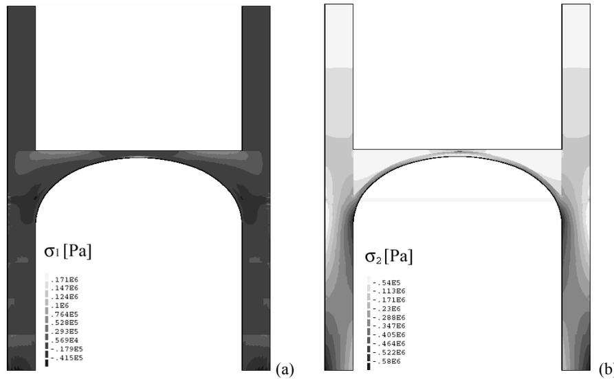
Figure 7 : (a) Structural analysis of the vault subjected to the dead load. Principal tensile stress contour; (b) principal compression stress contour, which emphasizes the shape of the thrust line.
