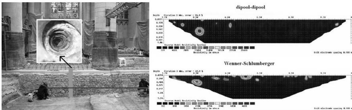
Figure 4 : left: black line = survey line; grey tube = borehole; right: dipole-dipole and Wenner-Schlumberger geo-electrical tomography showing the presence of the borehole.
