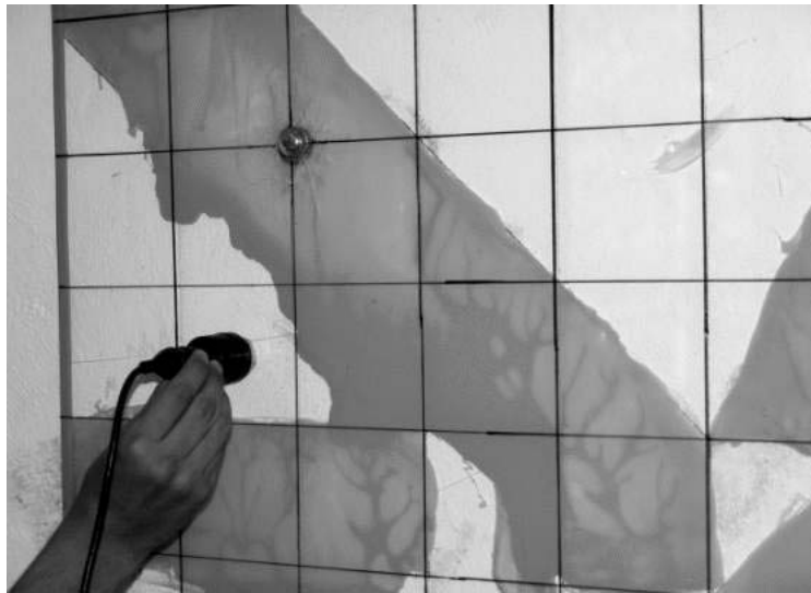
Figure 10 : Detail of dynamic testing of the laboratory specimen.
