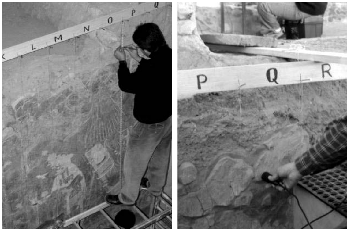
Figure 3 : Dynamic characterization process.
