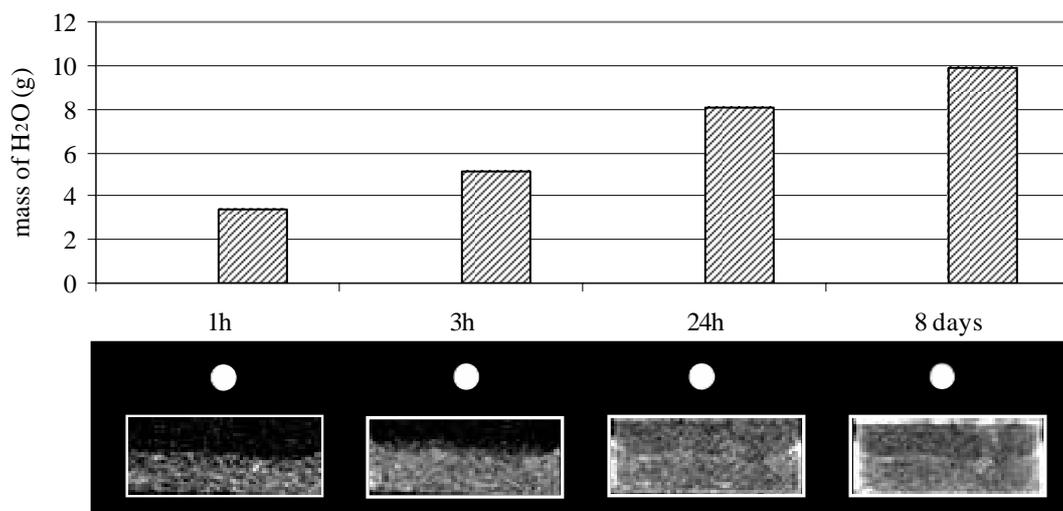
Figure 7 : MR images and mass determinations of the capillary water absorbed for a sample of Lecce stone treated with PB 72 by capillary absorption (190mg/100g of stone of active product) after different times of absorption. The upper face is the treated one.
