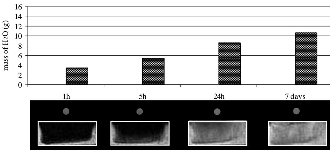
Figure 8 : MR images and mass determinations of the capillary water absorbed for a sample of Matera stone treated with PB 72 + W-OH by brush (497mg/100g of stone of PB 72 and 388mg/100g of stone of silica gel) after different times of absorption. The upper face is the treated one.
