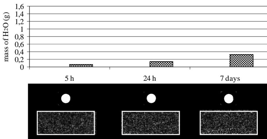
Figure 4 : MR images and mass determinations of the capillary water absorbed for a sample of travertine treated with ethyl silicate by brush (164mg/100g of stone of active product) after different times of absorption. The upper face is the treated one.
