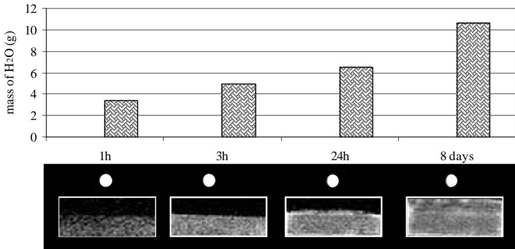
Figure 5 : MR images and mass determinations of the capillary water absorbed for a sample of Lecce stone treated with ethyl silicate by brush (814mg/100g of stone of active product) after different times of absorption. The upper face is the treated one. The lower face was placed in contact with liquid water.
