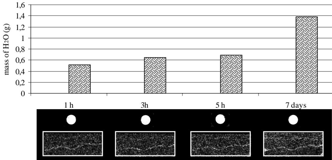
Figure 1 : MR images of a section within a sample of travertine and mass determinations of the water absorbed after different times of capillary water uptake. The lower face was placed in contact with liquid water. Brighter zones indicate higher detectable proton densities.
