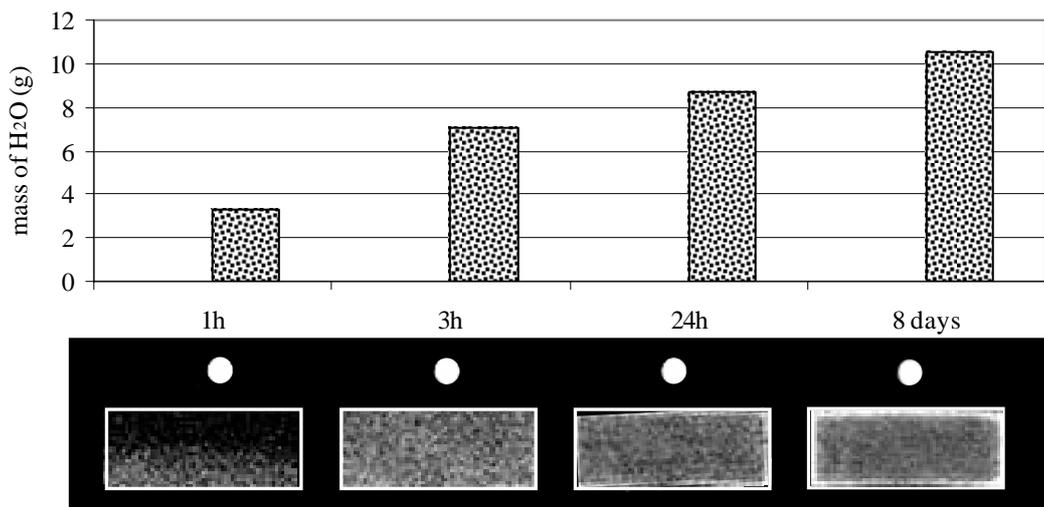
Figure 6 : MR images and mass determinations of the capillary water absorbed for a sample of Lecce stone treated with PB 72 by brush (74mg/100g of stone of active product) after different times of absorption. The upper face is the treated one.
