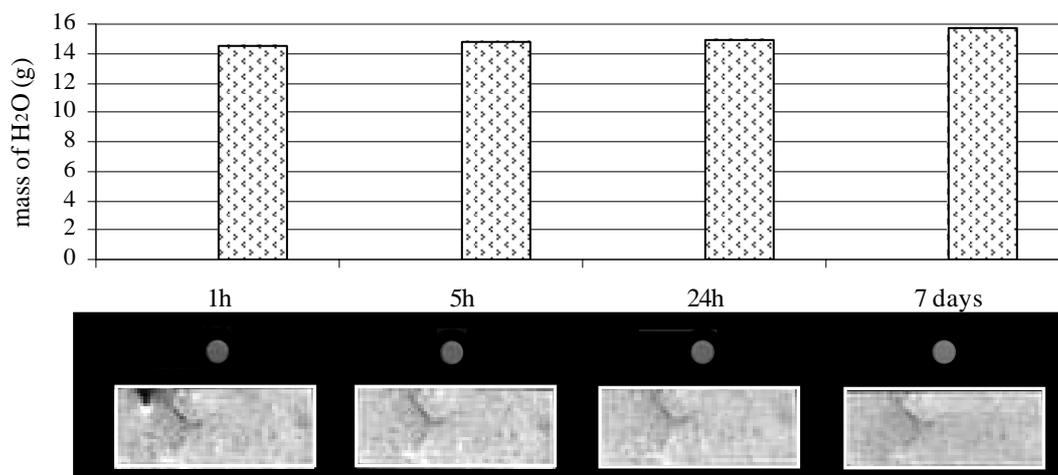
Figure 3 : MR images of a section within a sample of Matera stone and mass determinations of the water absorbed after different times of capillary water uptake. The lower face was placed in contact with liquid water.
