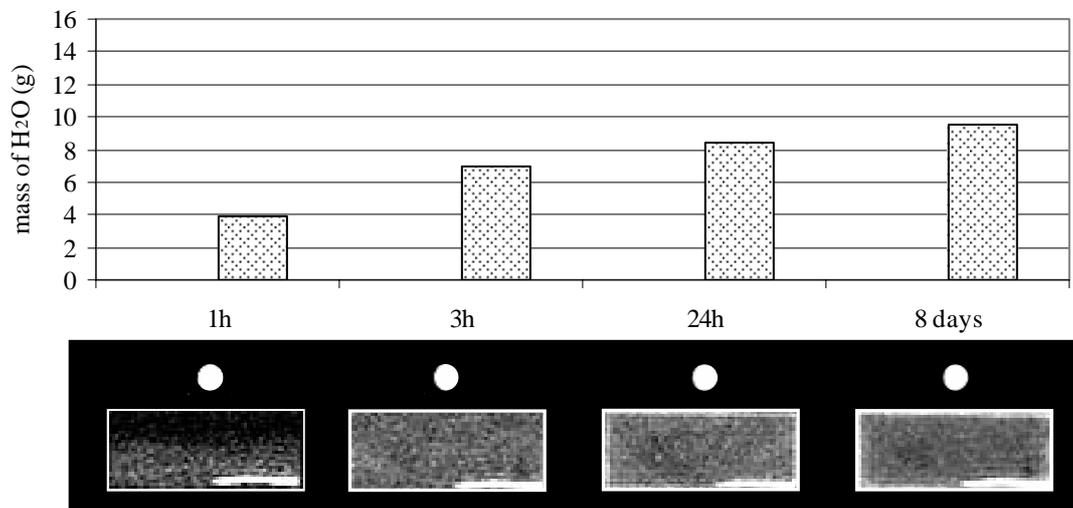
Figure 2 : MR images of a section within a sample of Lecce stone and mass determinations of the water absorbed after different times of capillary water uptake. The lower face was placed in contact with liquid water.
