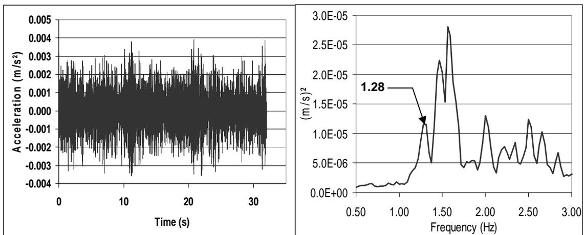
Figure 4 : Acceleration time record (left) and acceleration autospectrum (right)
