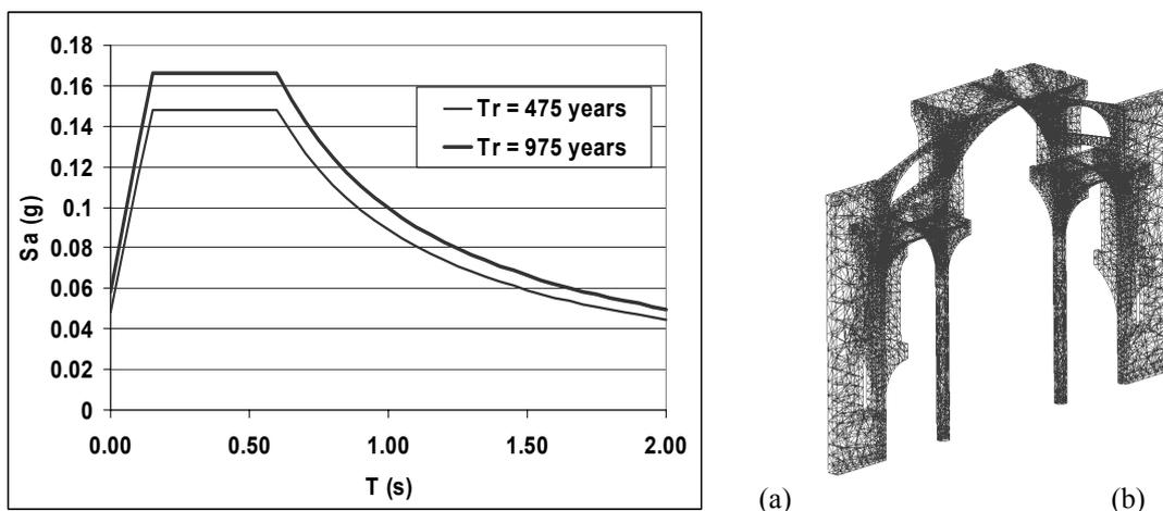
Figure 7 : (a) Elastic demand spectrum for 475 and 975-year return period; (b) FEM model
