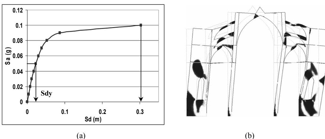
Figure 8 : (a) Capacity spectrum; (b) distribution of tensile damage at ultimate condition
