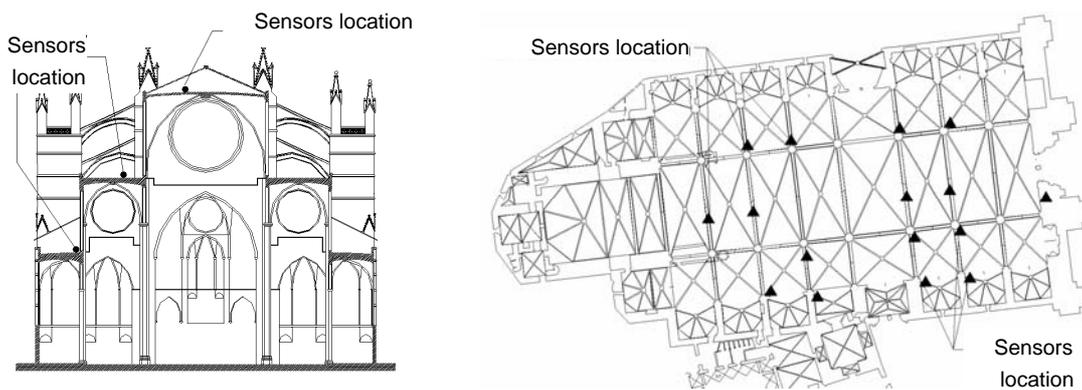
Figure 3 : Sensor location on a transversal section (left), and plan view sensors location (right)
