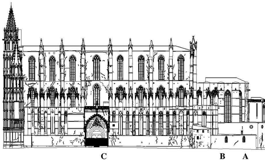
Figure 2 : Crack pattern of southern façade
