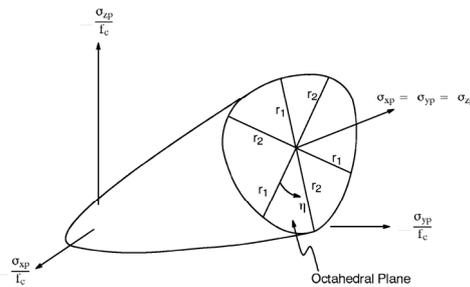
Figure 8 : Willam and Warnke failure surface
