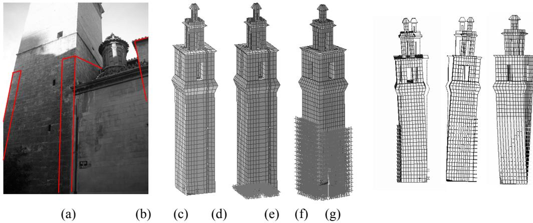
Figure 7 : Buttress in the tower. (a) Finite elements model of the tower. 3D view (b) West-South; (c) South-East; (d) North-East. Dynamic analysis results
