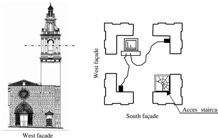
Figure 3 : West view. Accelerometers arrangement in the belltower.
