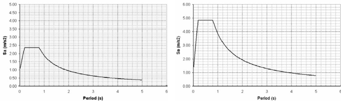
Figure 4 : Pseudo-acceleration spectrum. (a) Damping ratio 5%. (b) Damping ratio 1.59%
