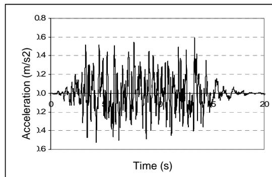
Figure 5 : Artificial accelerogram generated.
