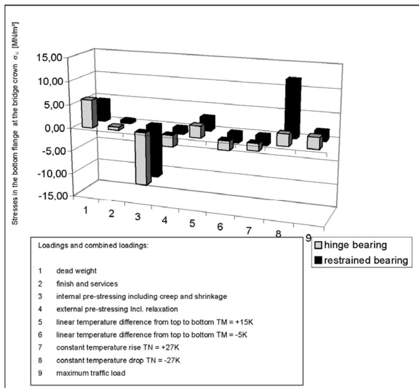
Figure 4 : Stresses in the bottom flange at bridge crown as caused by important loadings respective to the type of bearing.
