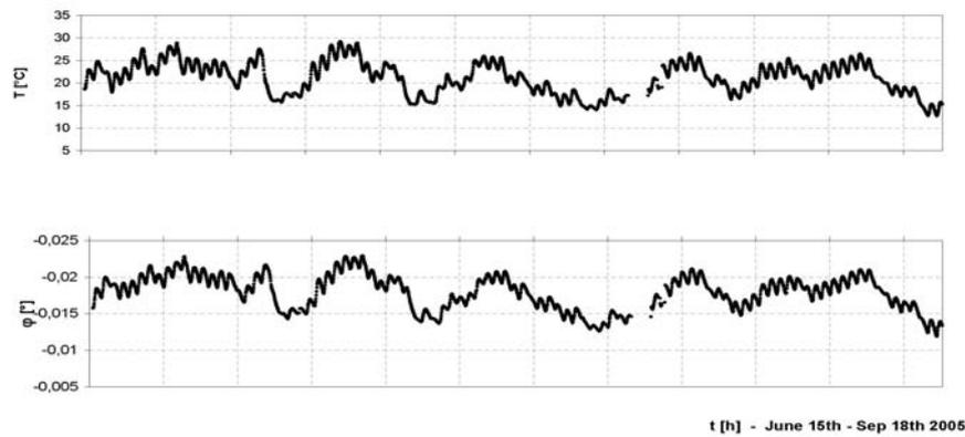
Figure 5 : Correlation between inclination at east portal frame leg and temperature in the bottom flange from June 15<sup>th</sup> to Sep 18<sup>th</sup> 2005
