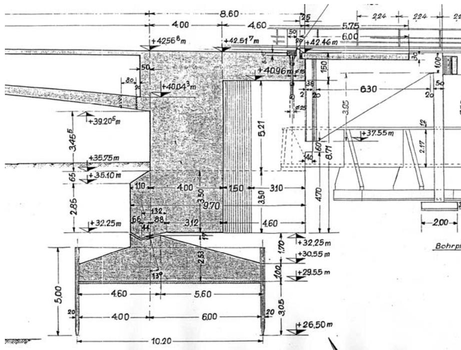
Figure 3 : Portal frame leg with hinge bearing, design drawing, 1957
