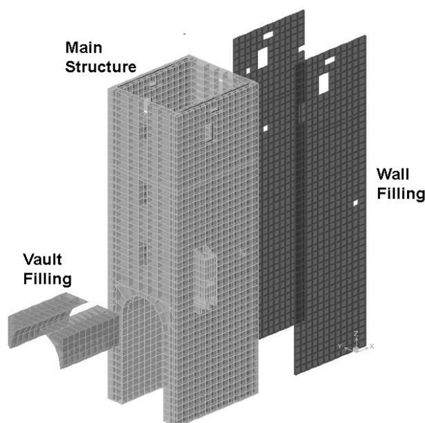
Figure 3 : FEM model of the Tower.
