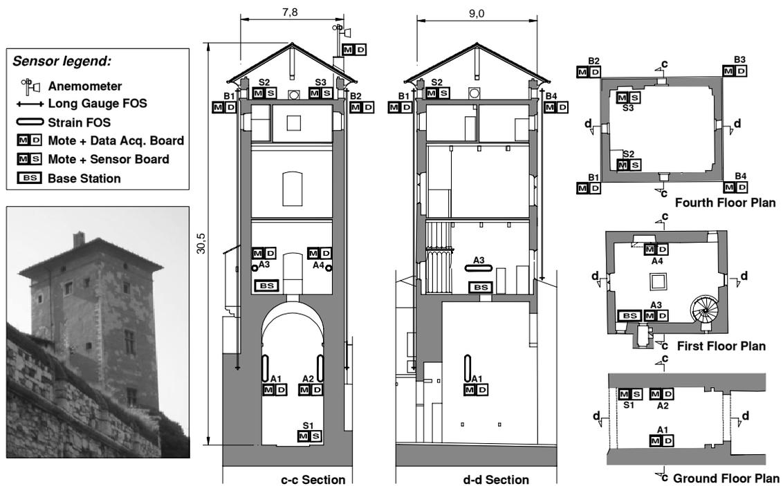
Figure 2 : Overview of the Tower; plan view and cross sections showing the instruments to be installed.
