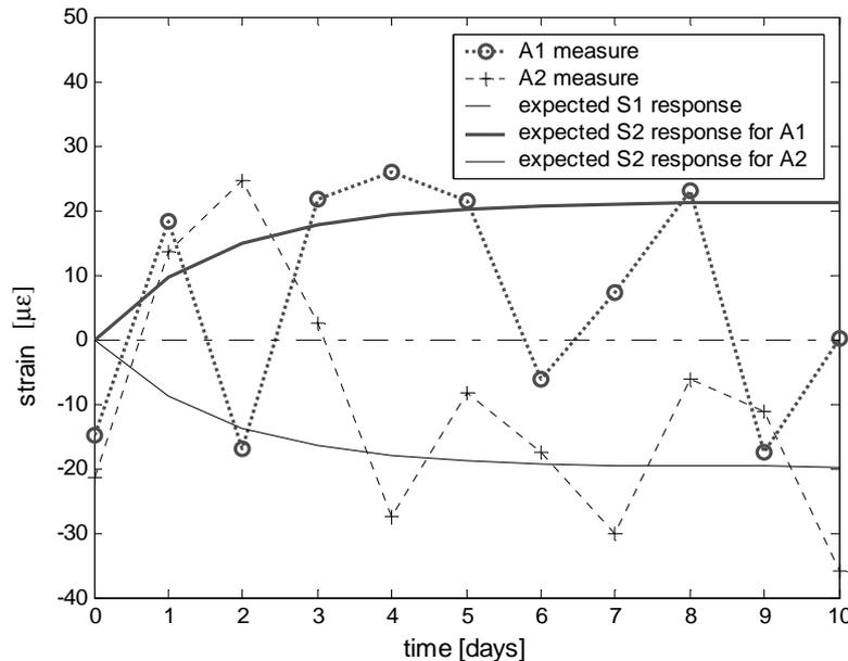
Figure 4 : Simulated measurements during subsidence, for sensors A1 and A2.
