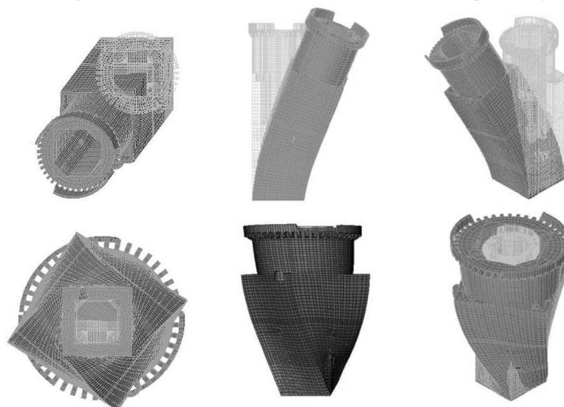
Figure 7 : First modal shape (1st flexural, top) and second modal shape (1st torsional, bottom) of the FEM model: plan, lateral view and axonometric view
