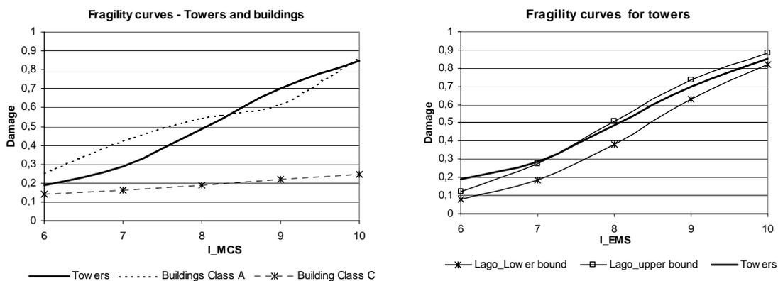
Figure 4 : Fragility curves for towers and ordinary buildings (left); correlation between expected average damage of the sample with the one formulated by Lagomarsino et al (2004) (right).
