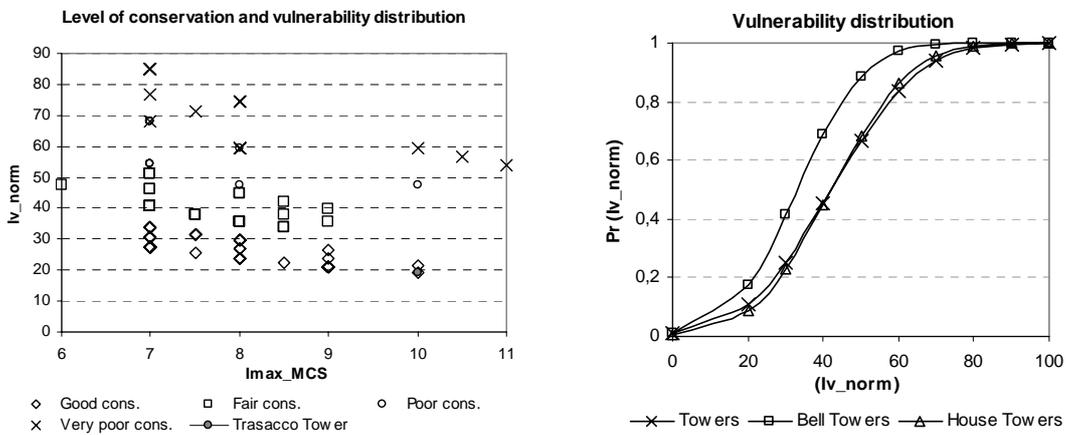
Figure 3 : Distribution of vulnerability of the sample using the speedy method of CNR-GNDT 2001
