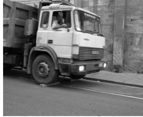
Figure 3 : Internal helical staircase; view from atop. Figure 4 : Impulsive excitation – calibrated lorry
