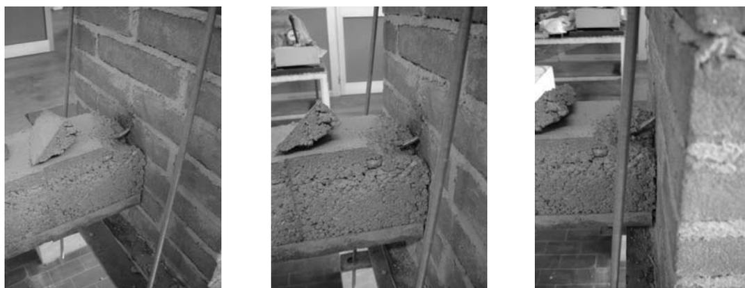
Figure 13,14,15 : Concrete failure at the connection
