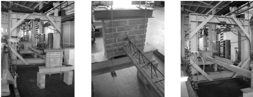
Figure 8,9,10 : Loading test on wall –floor connecting
