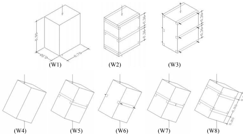
Figure 1 : Geometry of specimens: (W1)-(W3) tested in compression, (W4)-(W8) tested in diagonal compression.
