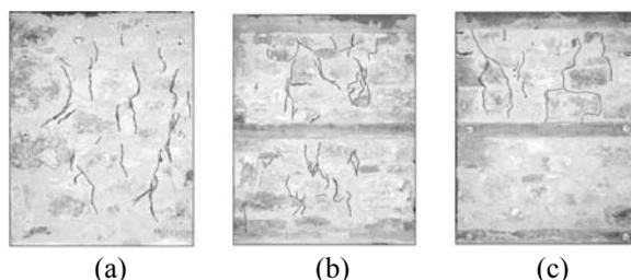
Figure 4 : Specimens tested in compression. Failure mode.
