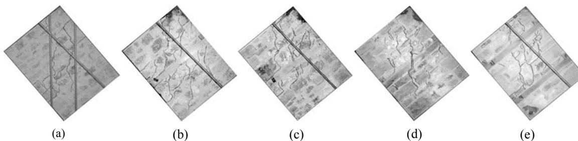
Figure 6 : Specimens tested in diagonal compression. Failure mode.
