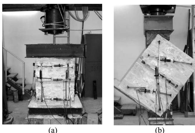
Figure 3 : Specimens to be subjected in (a) compression or in (b) diagonal compression, in their testing position.
