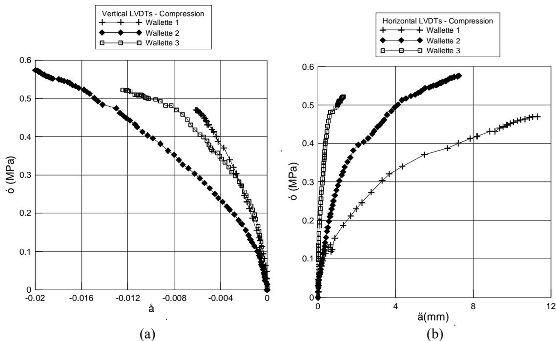
Figure 8 : Wallettes in compression, (a) Stress-strain curves, (b) stress-opening of vertical cracks
