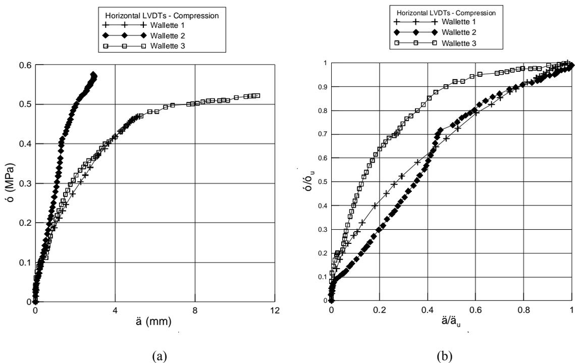
Figure 9 : Wallettes in compression, (a) vertical stress vs. opening of transverse cracks at mid-height, (b) normalized vertical stress vs. opening of transverse cracks curves at mid-height of the wallettes.
