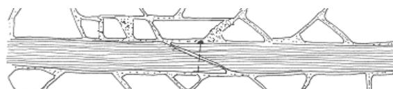
Figure 2 : The in-length connection of timber elements.
