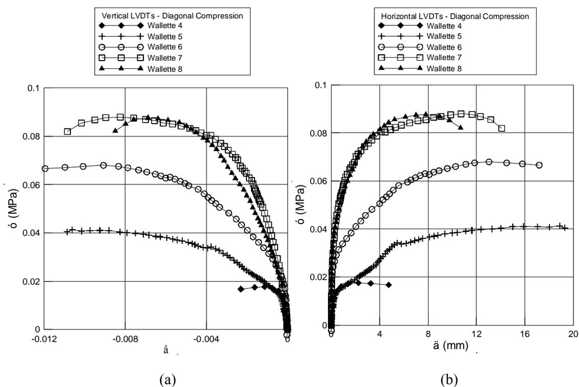
Figure 10 : Wallettes in diagonal compression, (a) Vertical stress-vertical strain curves, (b) Vertical stress-opening of vertical cracks curves.
