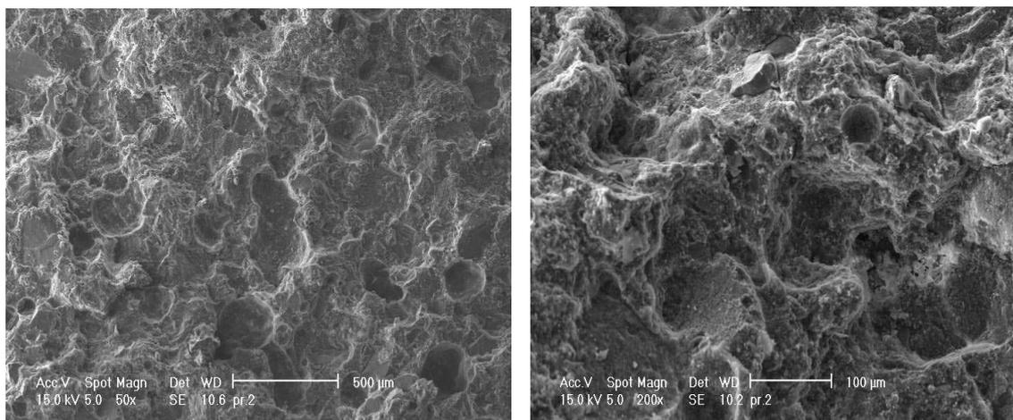
Figure 2 : SEM micrographs of historic mortars derived from the wall of the Kurzyniec Lock.
