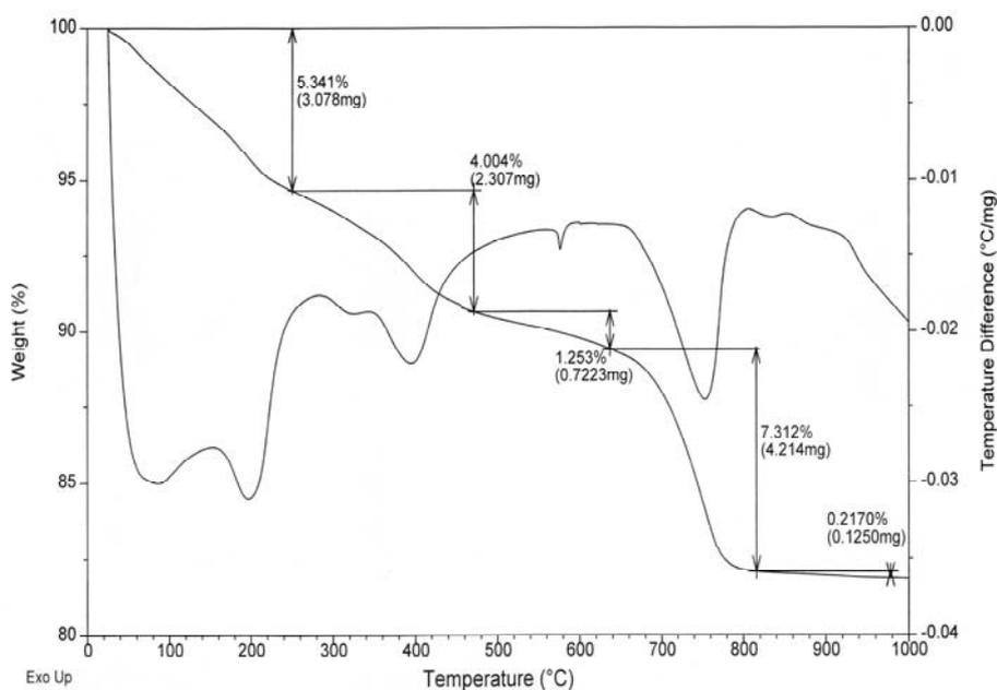
Figure 1 : Thermal analysis of P2 sample.
