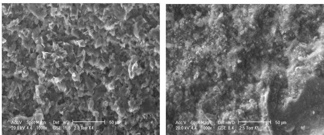
Figure 3 : E-SEM micrographs of mortars from the wall of the Kurzyniec Lock
