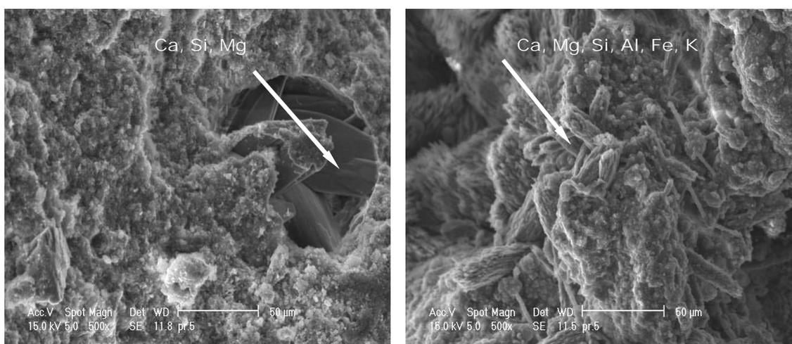
Figure 4 : SEM micrographs and EDS analysis of mortar of atypical morphology.
