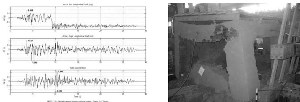
Figure 11 : M050-T11 phase 3. Acceleration response and model view after testing.
