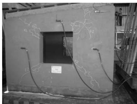
Figure 13 : Seismic behavior of model M080-E until phase 2. Hysteretic cycles and model view after testing.
