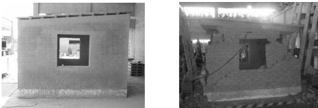
Figure 5 : Unreinforced Model M000 before the test (left) and after the test (right)
