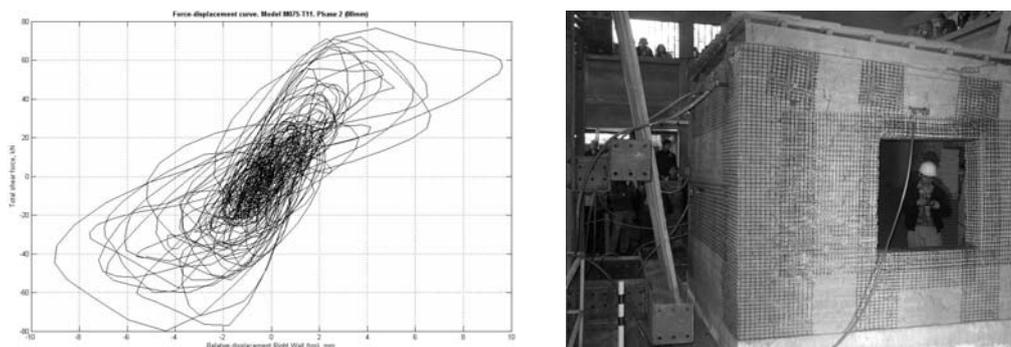
Figure 7 : Seismic behavior of model M075-T11 until phase 2
