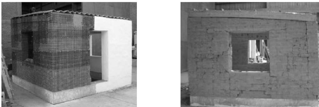
Figure 4 : Reinforced model M100-T12. Geogrid reinforcement and left wall after mesh removal.
