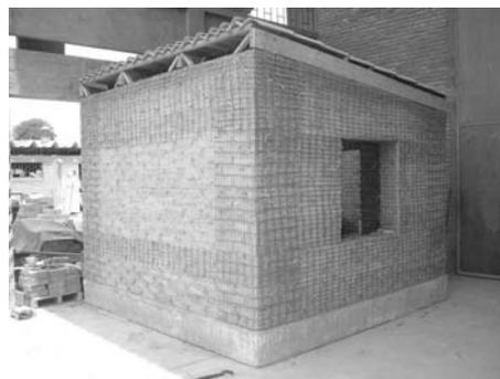
Figure 12 : Reinforcement arrangement and finished model M080-E.
