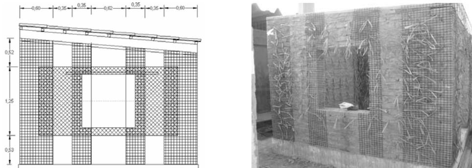
Figure 6 : Model M075-T11: reinforcement arrangement and model during construction.
