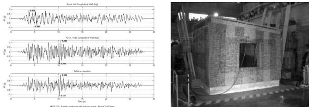
Figure 8 : Model M075-T11 phase 3. Acceleration response and model view after testing.
