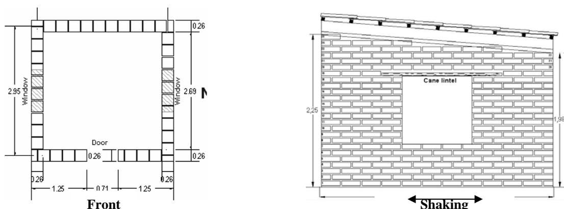
Figure 1 : Plan view and elevation of adobe models (Dimensions in m).
