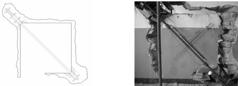
Figure 1 : Example of a diagonal compression test and cracking in the panel
