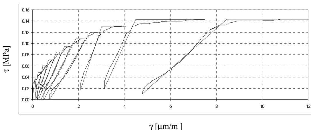
Figure 2 : Determination of the shear stiffness modulus for a Sillano panel
