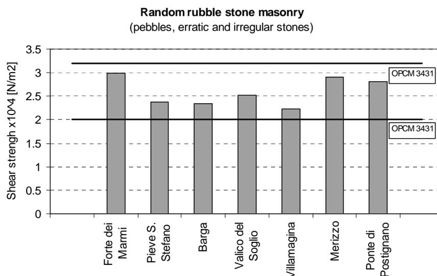
Figure 4 : Comparison between the experimental values and the threshold defined by the OPCM 3431
