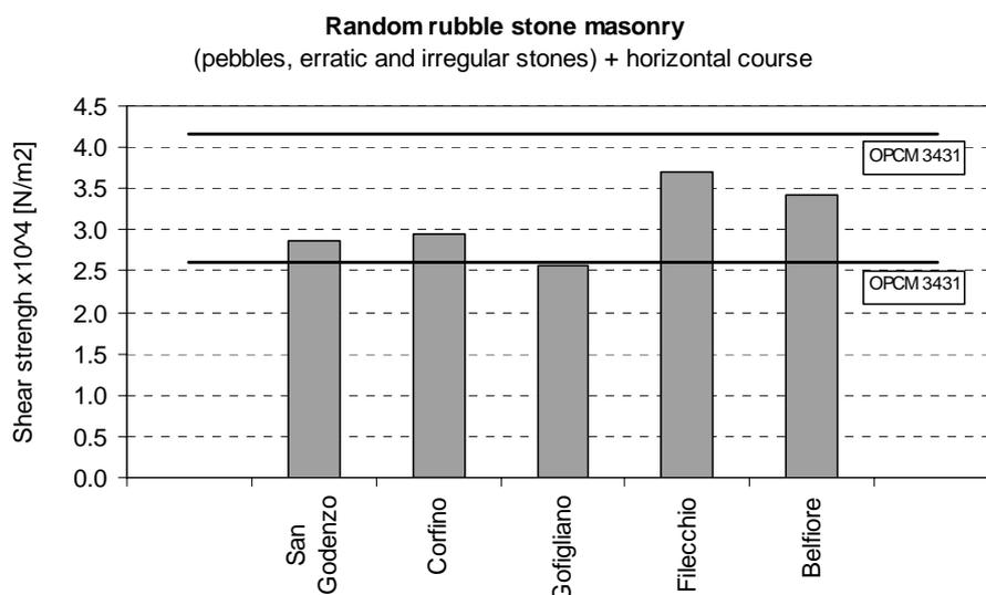
Figure 5 : Comparison between the experimental values and the threshold defined by the OPCM 3431
