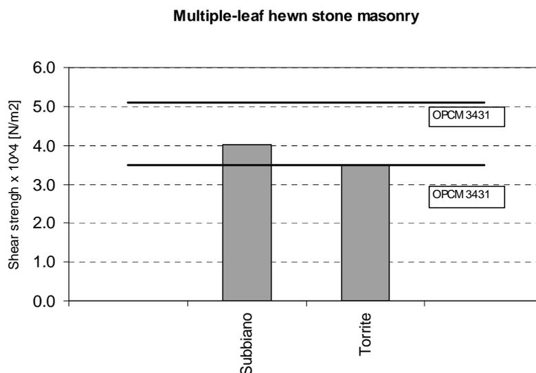
Figure 6 : Comparison between the experimental values and the threshold defined by the OPCM 3431
