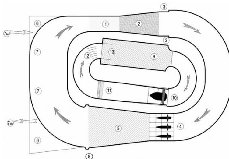
Figure 1 : Layout of the Jules Verne climatic wind tunnel at CSTB Nantes.
