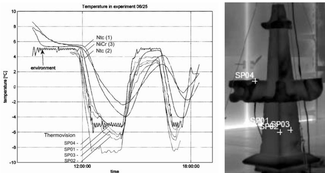
Figure 7 : Differences in surface temperature in the course of surrounding temperature cycle.
