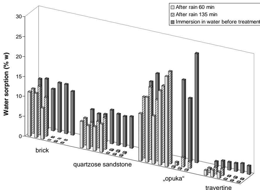
Figure 4 : Windy rain impact on brick and stone samples protected by water repellent and unprotected
