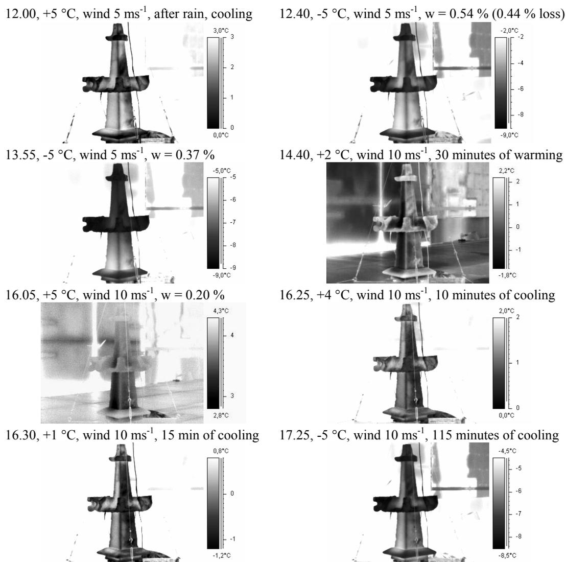
Figure 6 : Surface temperature changes on a previously wetted pinnacle with a hydrophobic coating subjected to cyclic temperature change and simultaneous wind flow.
