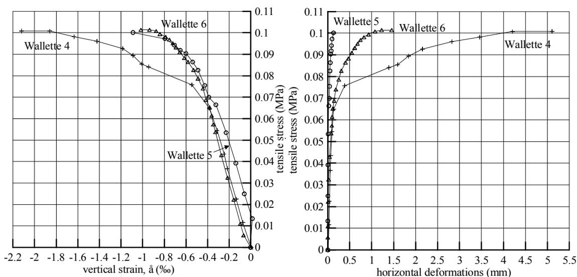
Figure 8 : Wallettes subjected to diagonal compression, (a) tensile strength-vertical strain curves, (b) tensile stress-horizontal deformation at mid-height of specimens
