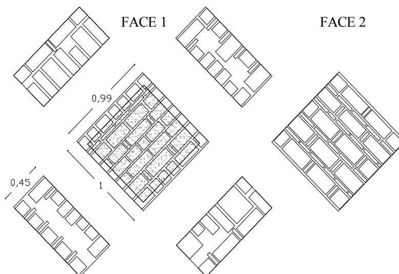
Figure 2 : Geometry of diagonal compression specimens.
