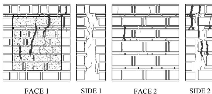
Figure 4 : Typical failure mode of wallettes in compression; Wallette 3
