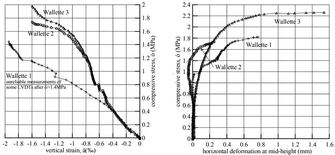
Figure 5 : Wallettes 1 to 3, (a) Vertical stress-vertical strain curves, (b) Vertical stress-horizontal deformations at mid-height of the specimens
