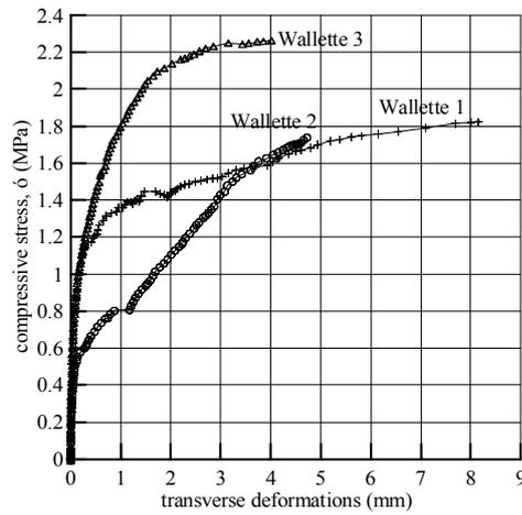
Figure 6 : Transverse deformations of Wallettes 1 to 3, subjected to compression
