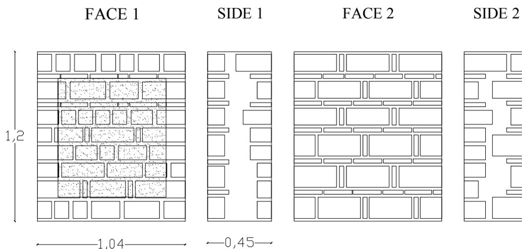
Figure 1 : Geometry of compression specimens (dimensions in [m]).
