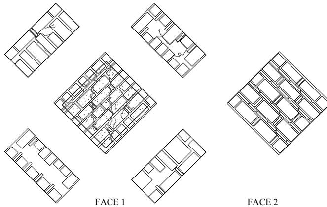
Figure 7 : Typical failure mode of specimens subjected to diagonal compression: Wallette 4.
