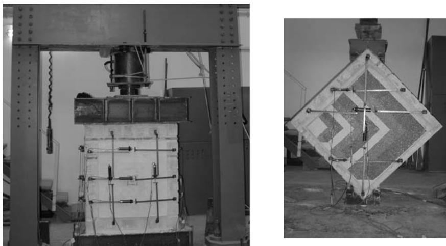
Figure 3 : Test set up for wallettes in compression and in diagonal compression.
