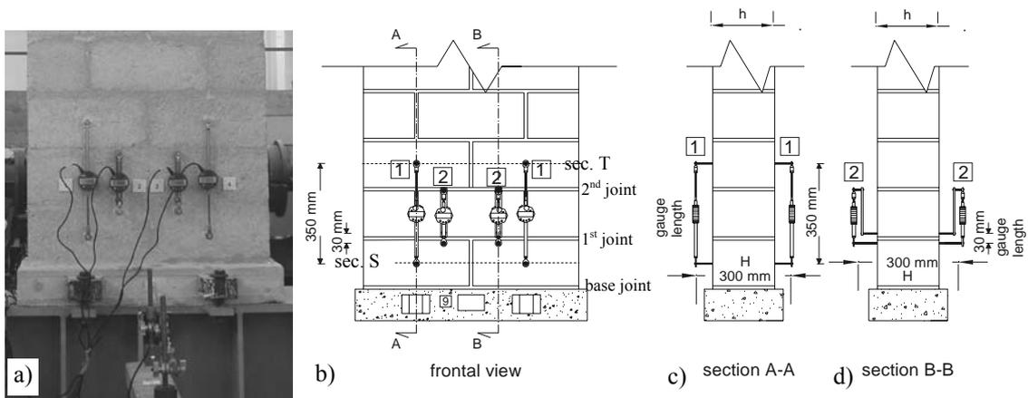
Figure 4 : Displacement transducers at the wall base: frontal view (a and b); lateral view (c and d).
