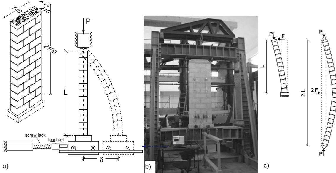
Figure 3 : Test specimen (a), test device (b) and equivalent loading schemes (c).
