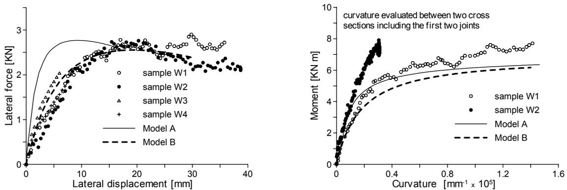
Figure 5 : Response of the walls: (a) lateral force against lateral displacement; (b) moment at the base cross-section against curvature evaluated between two cross sections including the first and the second joint.
