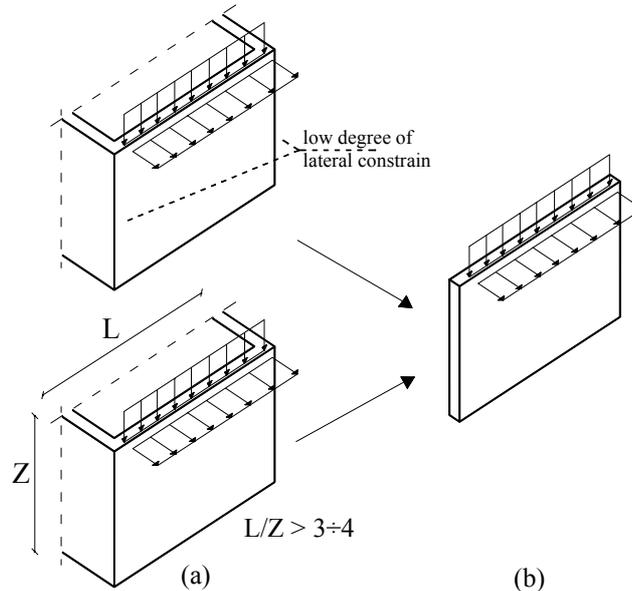
Figure 1: Examples of three-dimensional (a) and equivalent plane (b) schemes for analysis of walls.
