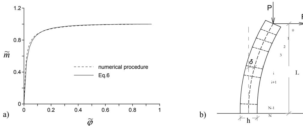
Figure 7: (a) Comparison between numerical and analytical moment-curvature law (b) and discretization of the wall for the evaluation of its global response.
