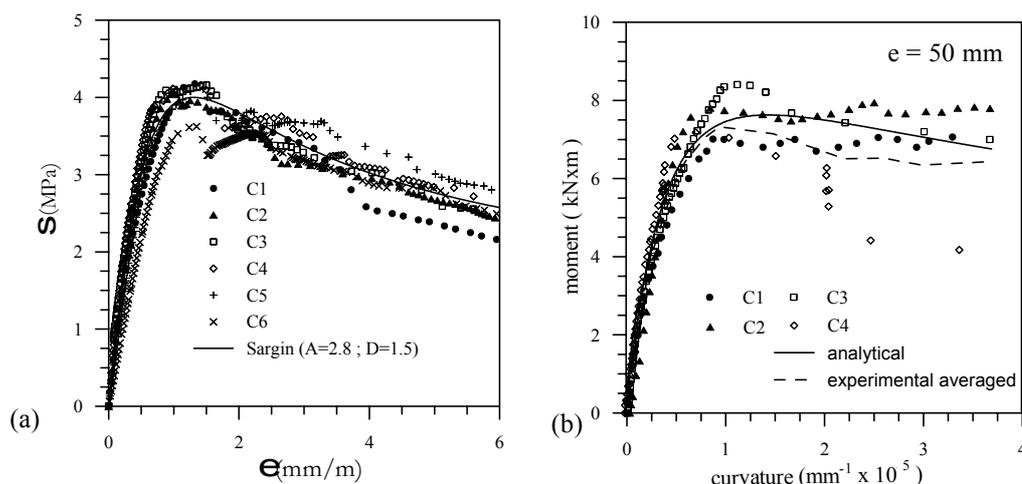
Figure 2 : Experimental and analytical stress-strain curves (a) and moment-curvature curves (b).
