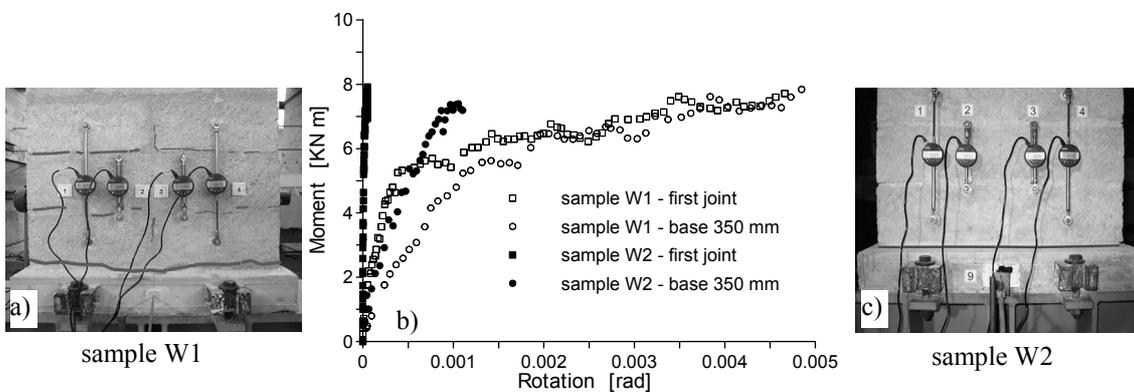
Figure 6 : Response of the walls: (a and c) distribution of the cracks at the base; (b) moments at the base cross-section against rotations.
