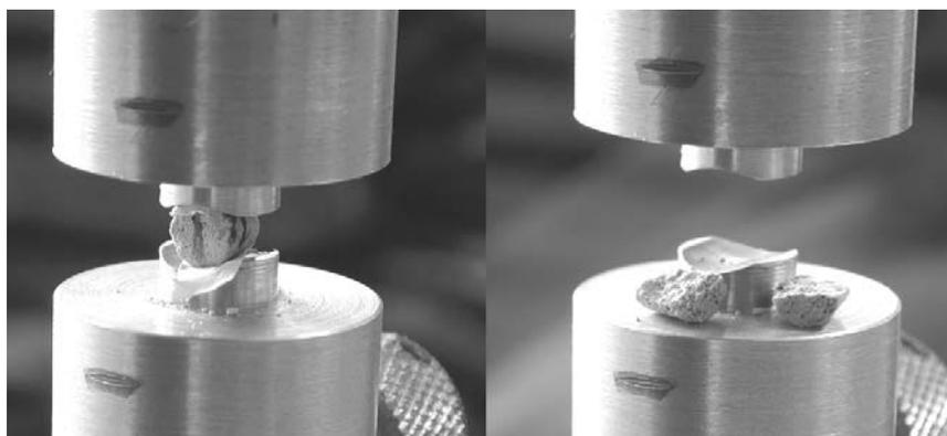
Figure 5 : Diametral compression of a micro-core and broken parts of the specimen.
