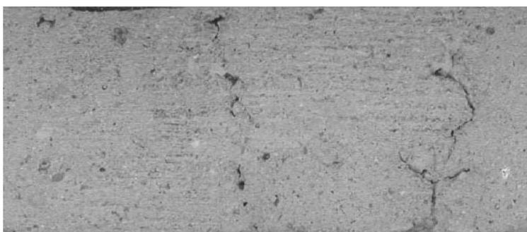
Figure 2 : Unwrapped surface of 6 mm brick micro-core with visible micro cracks and inclusions.
