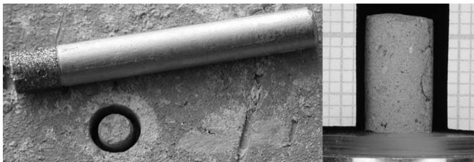
Figure 1 : Micro-core of 6 mm diameter in old brick and on a rotary table ready for image recording.
