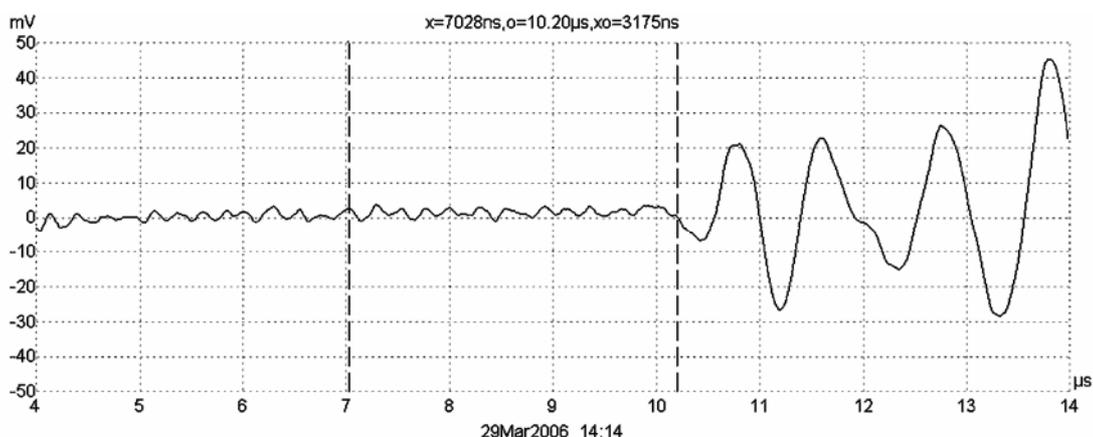
Figure 4 : Recorded longitudinal ultrasonic wave of 1 MHz in PW5b micro-core of length 6.04 mm.
