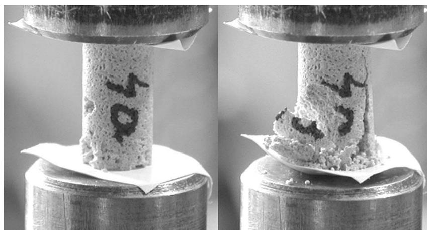
Figure 6 : Uniaxial compression of a slender cylinder. Specimen's dimensions are:  $d = 6.03 \text{ mm}$ ,  $h = 12.08 \text{ mm}$ .
