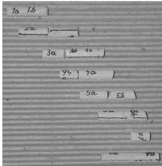
Figure 3 : Set of micro-cores of Portland Whitbed limestone after three point bending tests.
