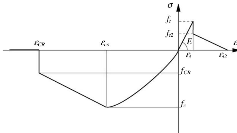
Figure 8 : Stress-strain relationship for masonry constitutive model
