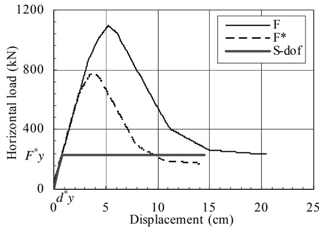
Figure 9 : Relationship between horizontal load and displacement determined by Pushover analysis
