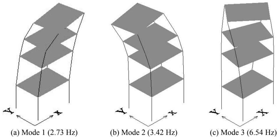
Figure 4 : Identification of the mode shapes
