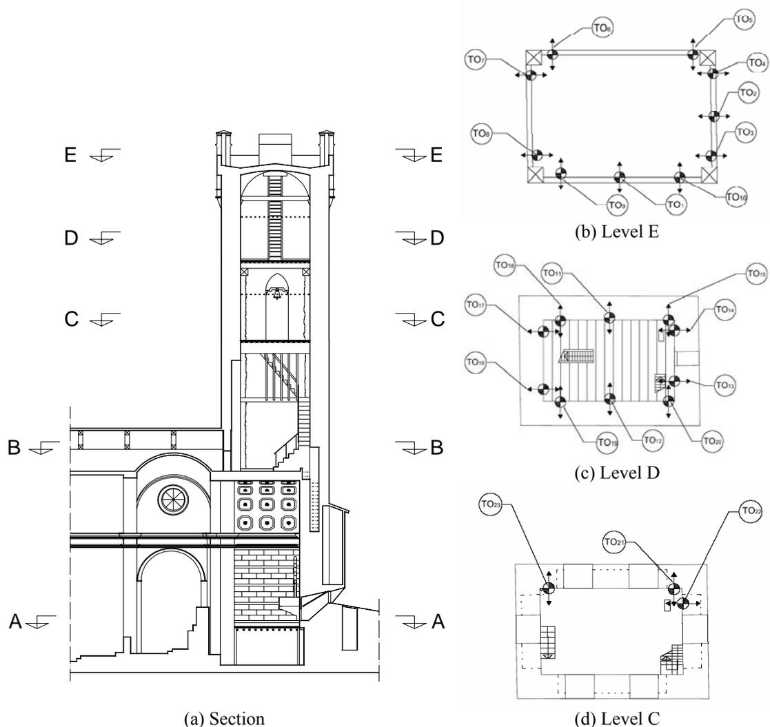
Figure 2 : Section and plan of Tower of Matilde and measuring points
