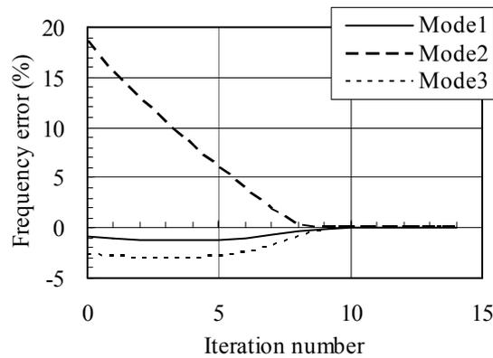
Figure 6 : Development of frequency error in iterative computation
