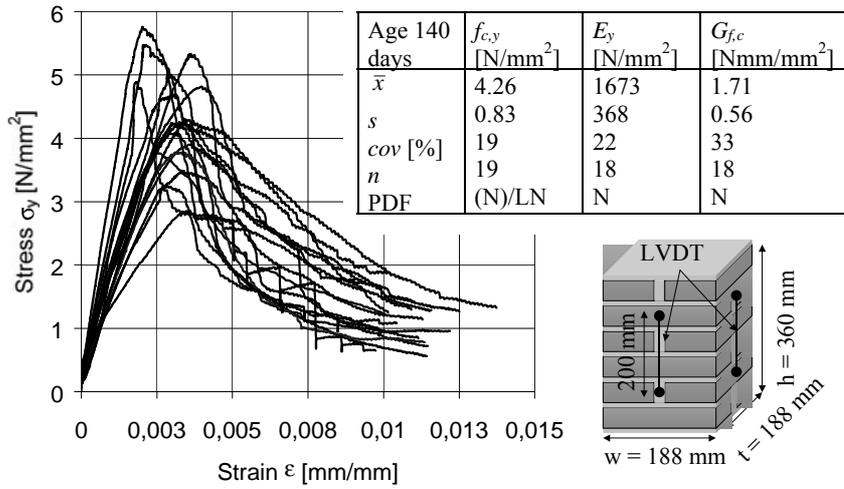
Figure 1 : Masonry pillars – stress-strain relationship and statistical summary
