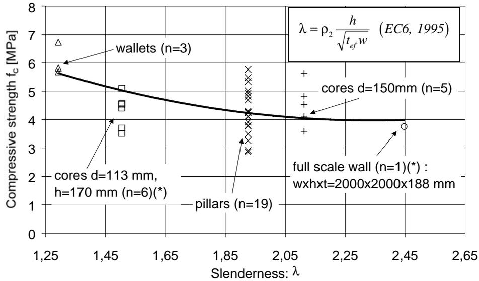
Figure 4 : Compressive stress versus slenderness
