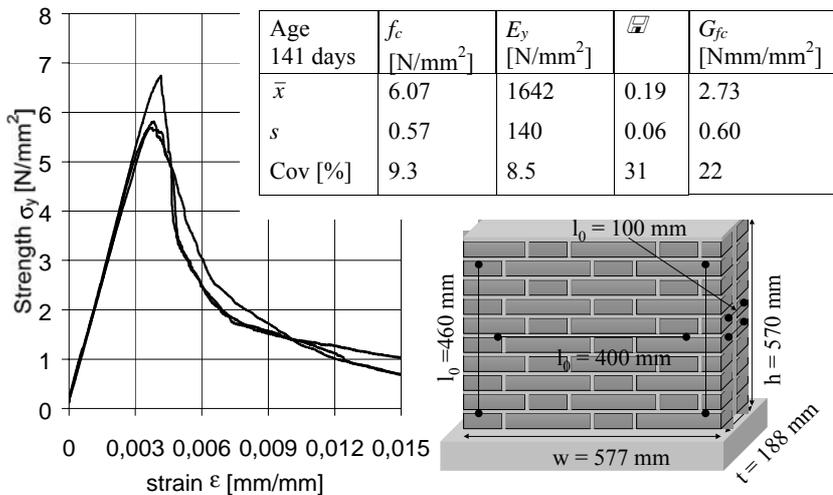
Figure 3 : Masonry wallets – stress-strain relationship and statistical summary
