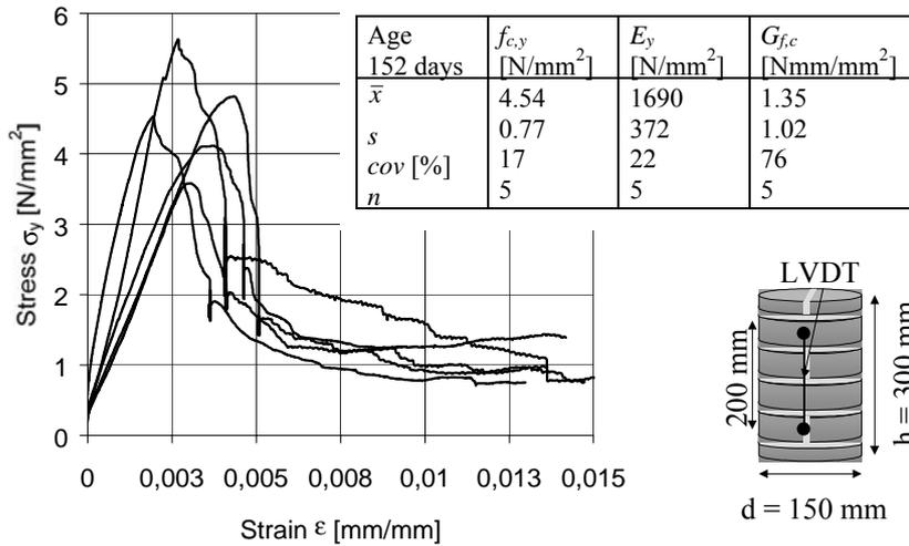
Figure 2 : Masonry cores-stress-strain relationship and statistical summary
