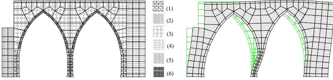
Figure 4: Left: rigid element model with indication of the 6 different materials assigned to the elements. Right: deformed shape corresponding to the first natural mode of vibration, at 4.8 Hz.
