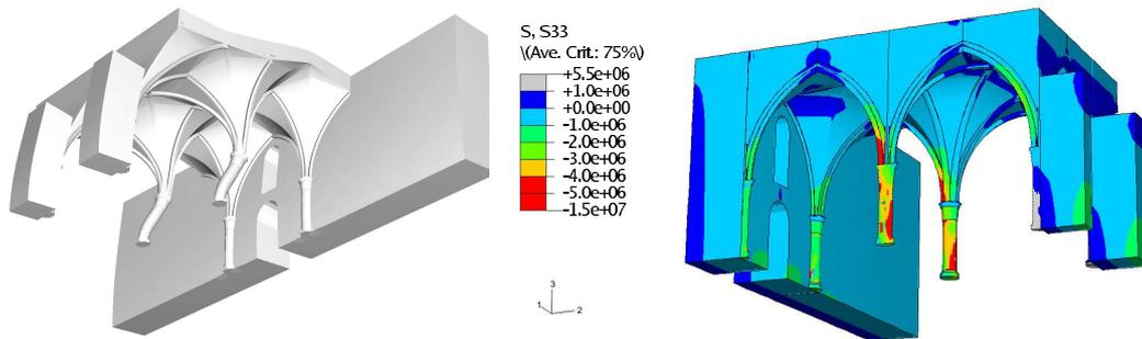
Figure 3: Deformed shape of the first natural mode of vibration of the detailed model of the hypostyle chamber (left) and distribution of the vertical axial stress  $S_{33}$  [Pa] caused by the action of gravity plus a lateral acceleration equal to  $2.5 \text{ m/s}^2$  (right).
