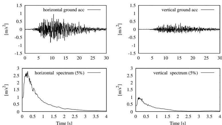
Figure 7: The accelerograms and their elastic response spectrum at 5% of damping.
