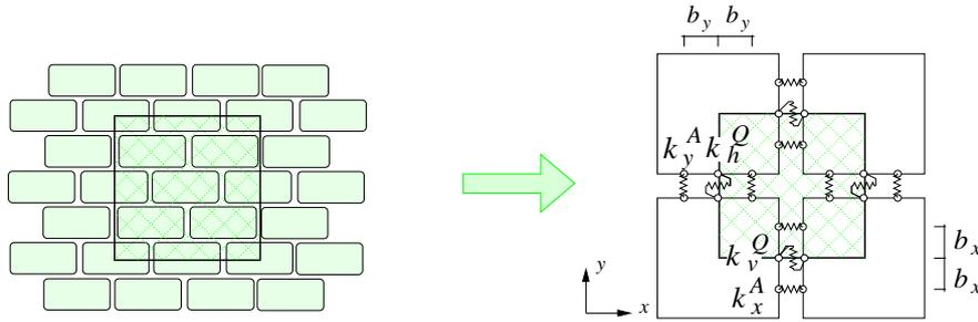
Figure 1: Scheme of a regular masonry texture and an example of “unit cell” made of rigid elements connected by line springs.
