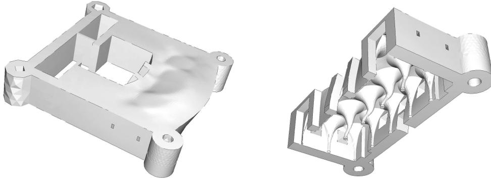
Figure 2: Deformed shape of the first natural mode of vibration of the whole castle.
