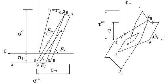
Figure 6: Hysteretic behaviour for the axial (left) and shear (right) connecting springs.
