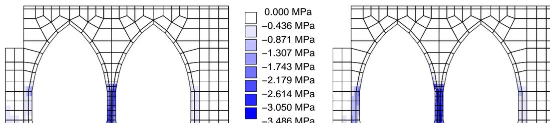
Figure 10: Vertical axial stress *before* (left) and *after* (right) the seismic loading.
