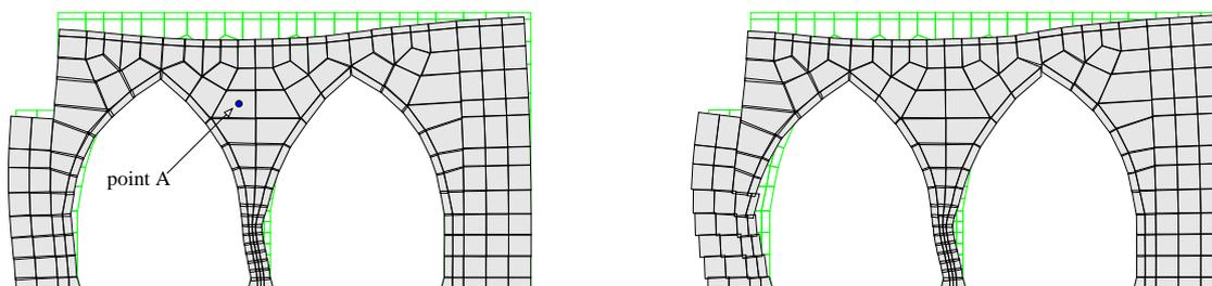
Figure 9: Deformed shape *before* (left) and *after* (right) the seismic loading.
