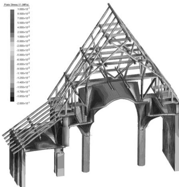
Figure 8 : Global model with the roof: axial stresses (hypothesis of hinged supports at the bases)
