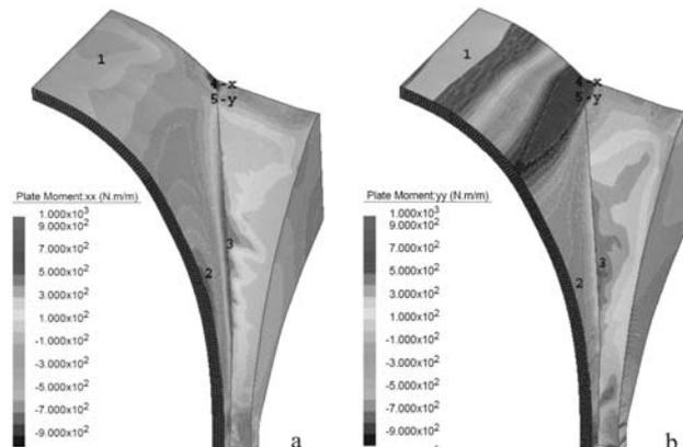
Figure 13 : Bending stresses; (a) X and (b) Y direction. Detail model. Repaired state.
