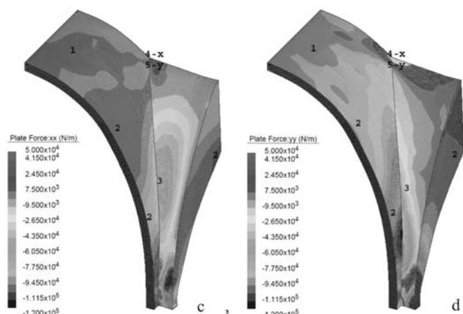
Figure 14 : Axial stresses; (c) X and (d) Y direction. Detail model. Repaired state.
