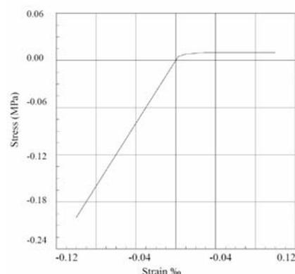
Figure 10 : Non linear behaviour of the material
