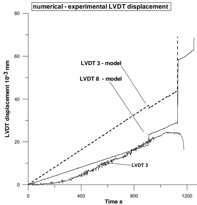
Figure 8 : Specimen PN2: experimental LVDT vertical displacement and numerical modeling at the failure of the first connection
