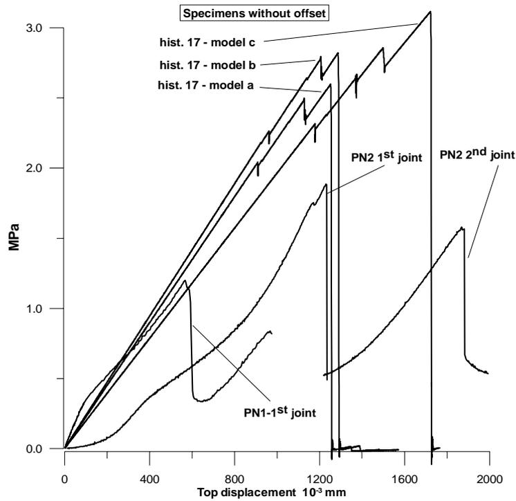
Figure 7 : Noto stone without offsets: specimens PN1 and PN2
