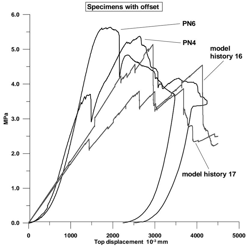
Figure 3 : Noto stone with offset – specimens PN4 and PN6
