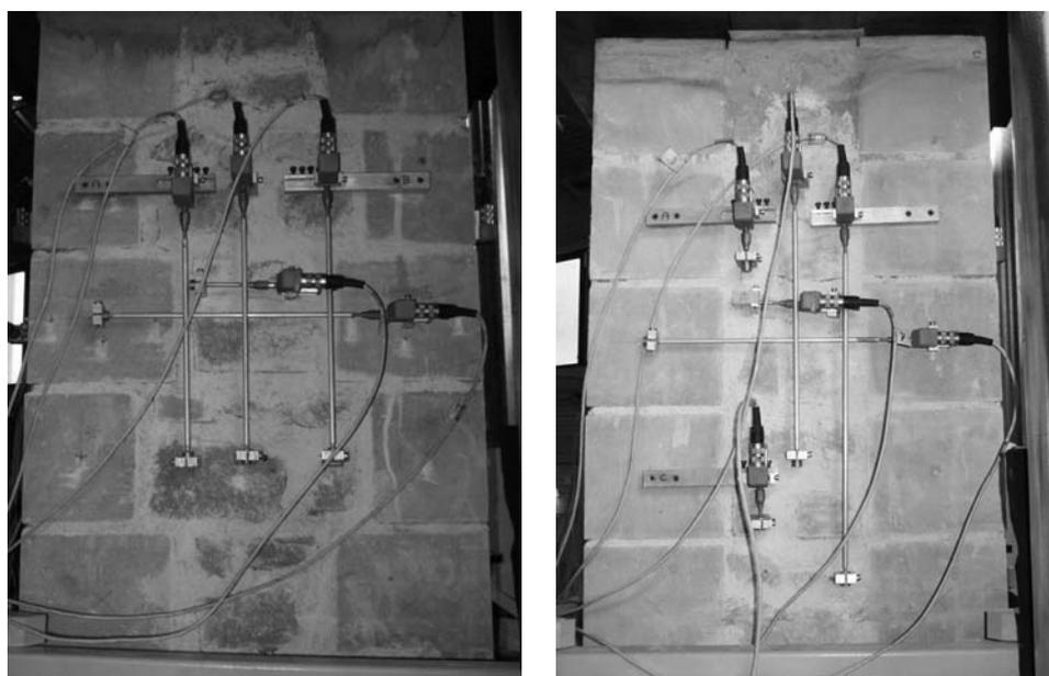
Figures 1, 2 : Specimens with and without offsets: displacement transducers position.
