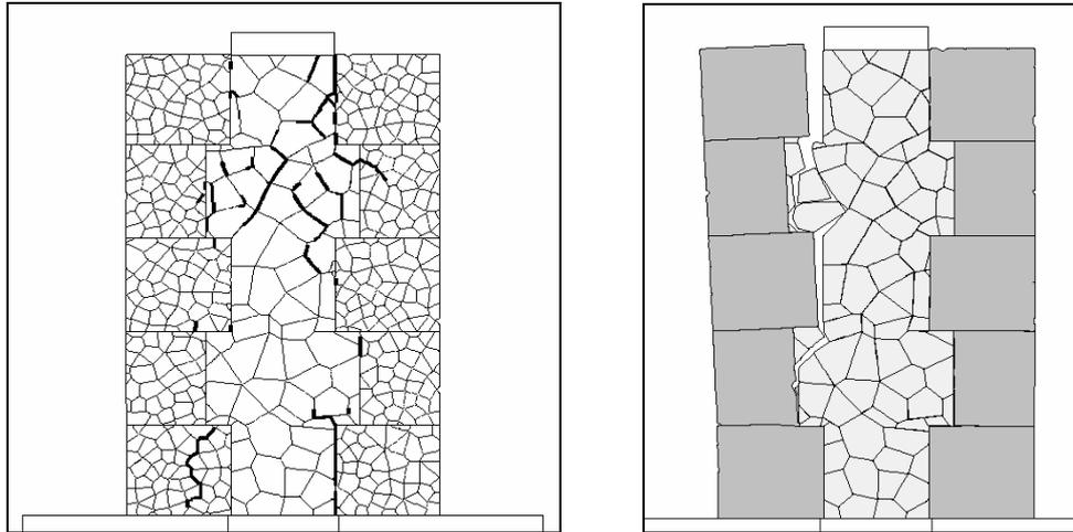
Figures 5, 6 : Fracture modeling in blocks at 3.5 mm top displacement and collapse modeling of the specimen, at large displacements.
