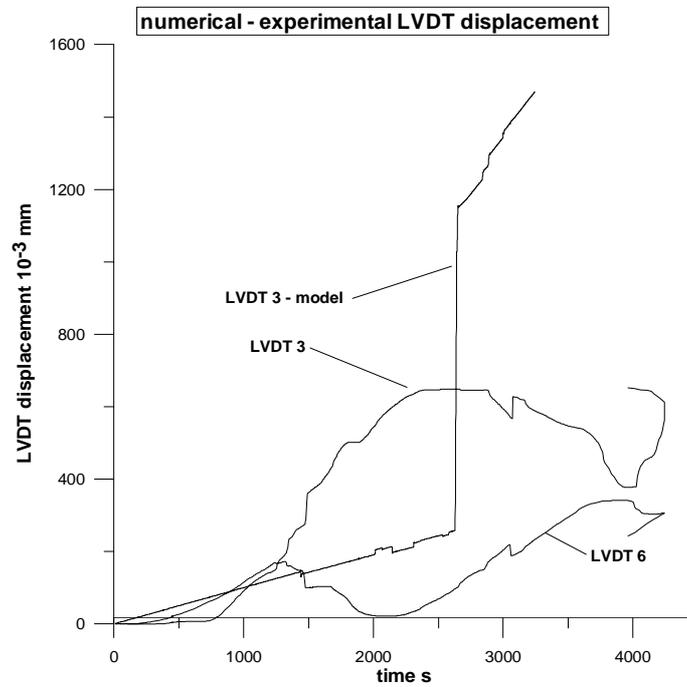
Figure 4 : Specimen PN4: experimental LVDT vertical displacement and numerical modeling
