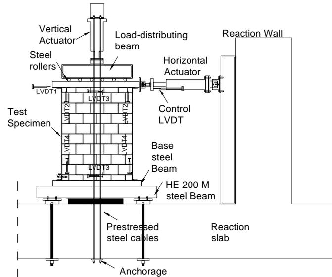
Figure 1: Experimental Test Set-Up and Position of LVDTs (Vasconcelos 2005)
