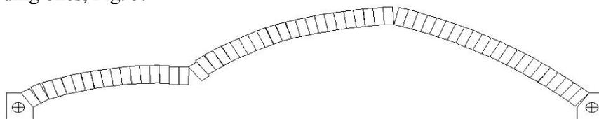
Figure 3 : Case (i) - Collapse mode of the Bridgemill bridge arch without fill for “line” live-load.
