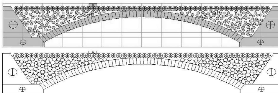
Figure 2 : Top) Unacceptable sub-domains for the CDE (gray) and rectangular reticulated mesh, Bottom) distribution of the CDE after the radius expansion stage.
