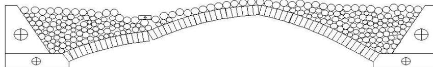
Figure 4 : Collapse mode of the arch with fill due to “line” live-load.
