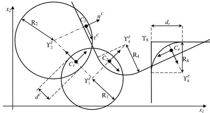
Figure 1: Representation of the contacts between several discrete elements.
