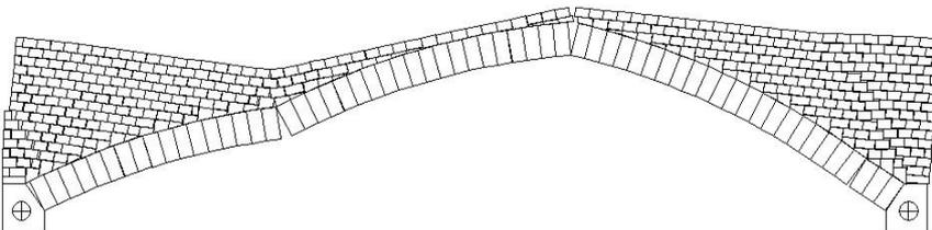
Figure 5 : Collapse mode of Bridgemill bridge arch with spandrel wall due to “line” live-load.
