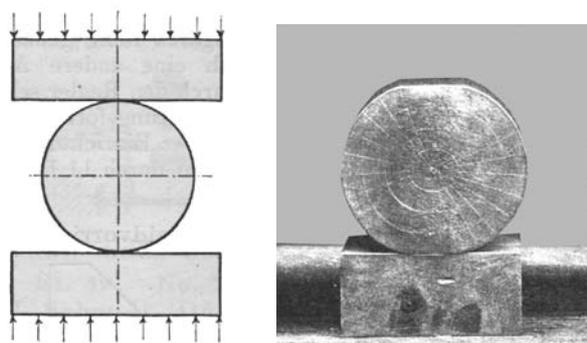
Figure 1 : Model showing flattenings in the contact area (Bach 1894)
