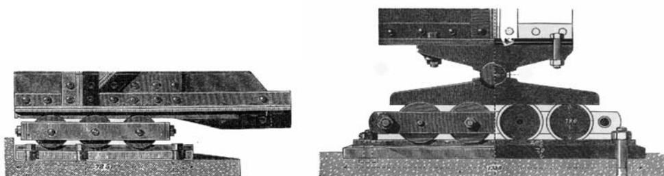
Figure 2 : Typical historical plane bearing (left) and rotating bearing (right) (Winkler 1875, p.271, 286)
