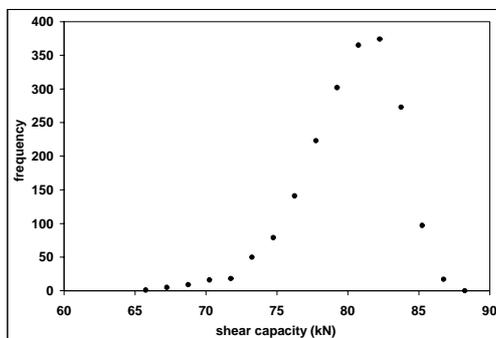
Figure 4 : Frequency distribution of shear capacity for the un-reinforced brick masonry wall
