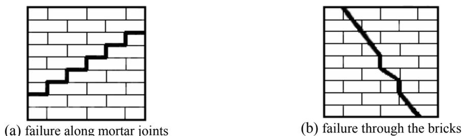
Figure 2 : Diagonal shear mode of failure
