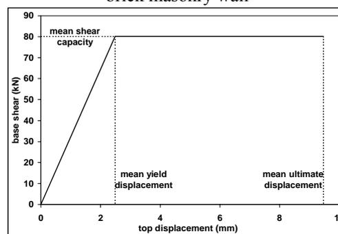
Figure 7 : Mean capacity curve for the un-reinforced brick masonry wall against in-plane loading
