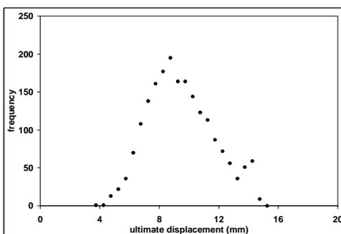
Figure 6 : Frequency distribution of ultimate displacement at the top of the un-reinforced brick masonry wall
