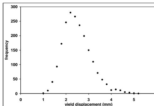
Figure 5 : Frequency distribution of yield displacement at the top of the un-reinforced brick masonry wall
