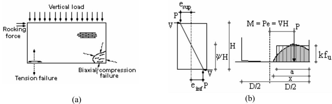
Figure 1 : Flexural/Rocking mode of Failure
