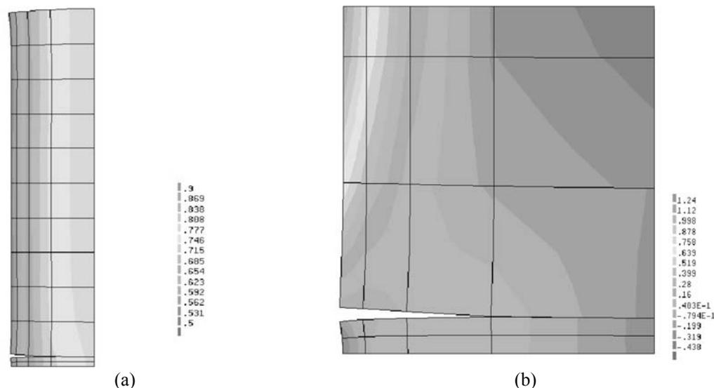
Figure 6 : (a) Moisture content and deformation pattern across the cross section; (b) detail stone-joint: resulting stress in y-direction and deformation pattern
