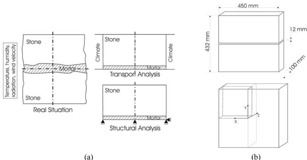
Figure 5 : (a) Geometric model and deformation conditions in the research model; (b) two-dimensional illustration for the wall cross section / Utilization of symmetries.
