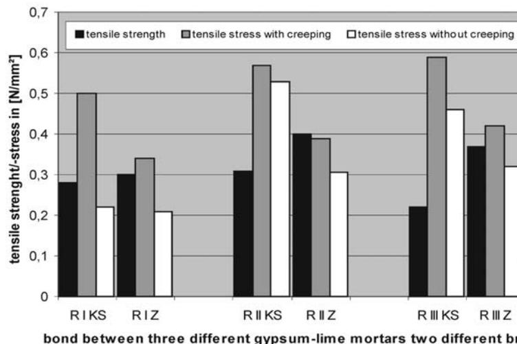
Figure 4 : Results of the calculation of flank cracking of different mortars and bricks.
