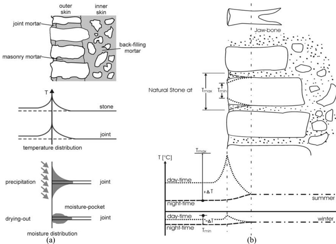
Figure 1 : (a) Thermal and hygric exposure of historical masonry; (b) deformation of natural stones in historical masonry as a result of thermal elongation.
