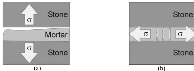
Figure 2 : (a) Cracking parallel to joint; (b) cracking normal to the joint.
