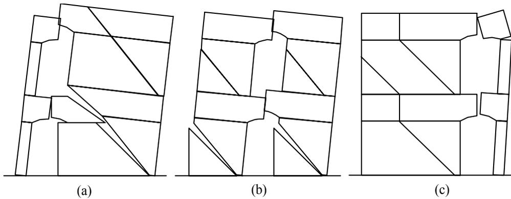
Figure 6 : Failure mechanisms for Macro-blocks 01 with (a)  $x/W = 0.2$ ; (b)  $x/W = 0.5$  and (c)  $x/W = 0.8$
