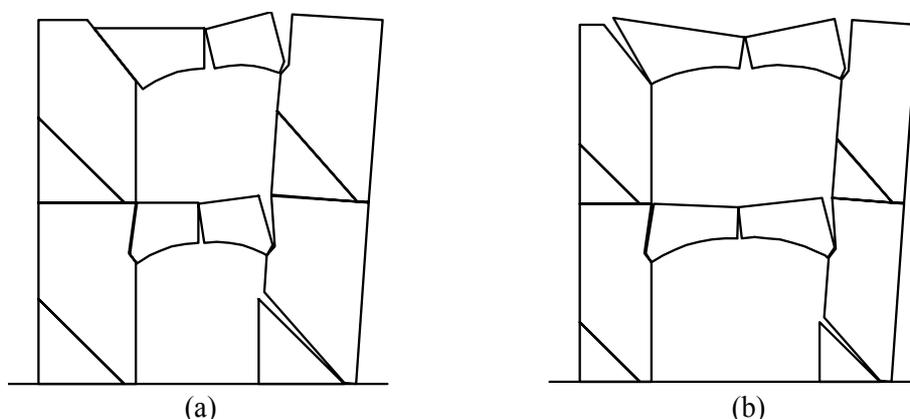
Figure 9 : Failure mechanisms for Macro-blocks 02 with (a)  $w/W = 0.38$  and (b)  $w/W = 0.53$
