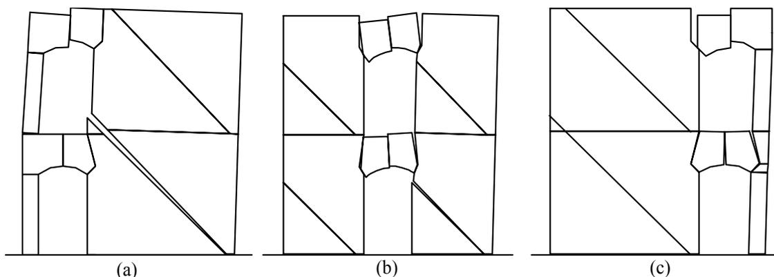
Figure 8 : Failure mechanisms for Macro-blocks 02 with (a)  $x/W = 0.2$ ; (b)  $x/W = 0.5$  and (c)  $x/W = 0.8$ .
