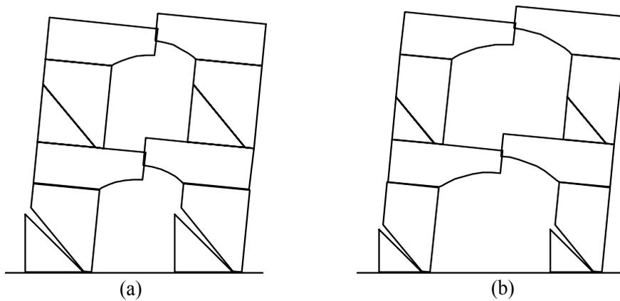
Figure 7 : Failure mechanisms for Macro-blocks 01 with (a)  $w/W = 0.38$  and (b)  $w/W = 0.53$
