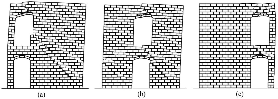
Figure 3 : Failure mechanisms for micro-blocks with (a)  $x/W = 0.2$ ; (b)  $x/W = 0.5$  and (c)  $x/W = 0.8$ .
