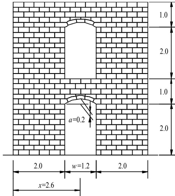
Figure 1 : Basic geometry of the micro-models.
