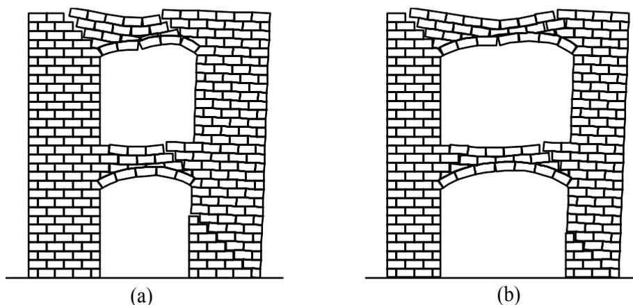
Figure 5 : Failure mechanisms for micro-blocks with (a)  $w/W = 0.38$  and (b)  $w/W = 0.53$ .
