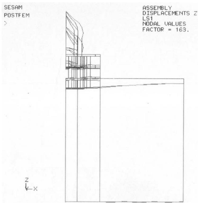
Figure 5 : Displacement,  $w$  in Z-direction for complete structure
