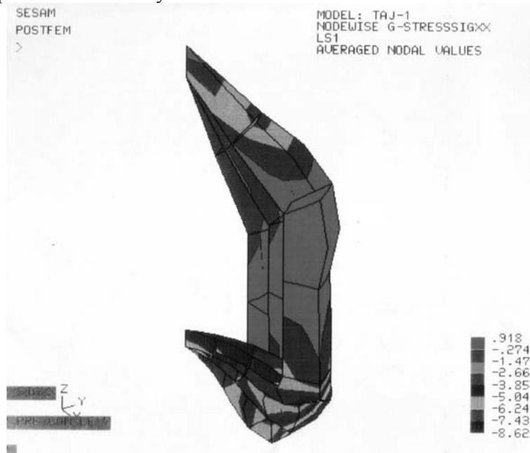
Figure 7.: Stress contours for  $\sigma_x$  in domical portion
