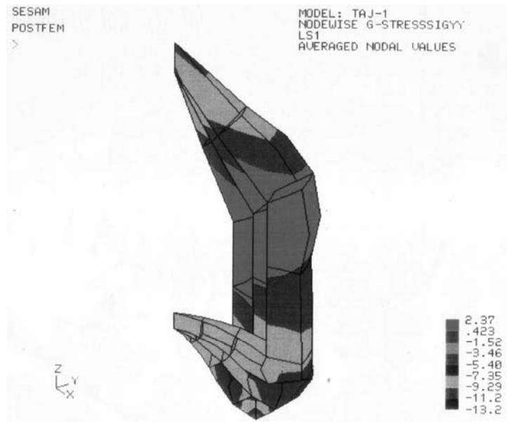
Figure 8 : Stress contours for  $\sigma_y$  in domical portion
