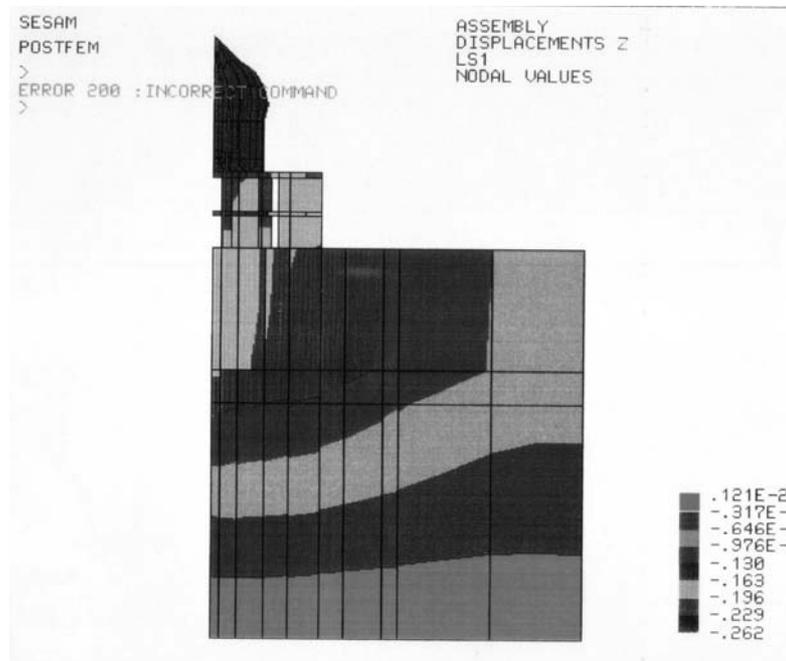
Figure 6 : Contours of vertical displacement,  $w$  in Z-direction for complete structure
