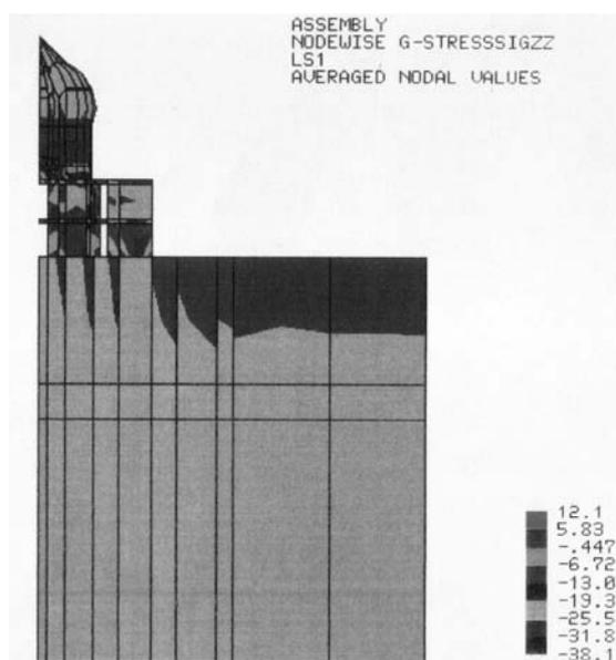
Figure 9 : Stress contours for  $\sigma_z$  in domical portion
