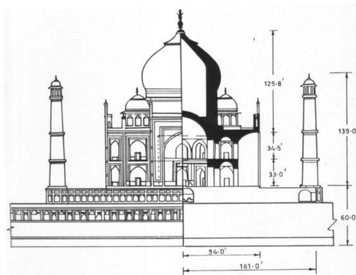
Figure 1 : Part elevation and part sectional elevation of the Taj Mahal (1 ft = 0.3048 m)
