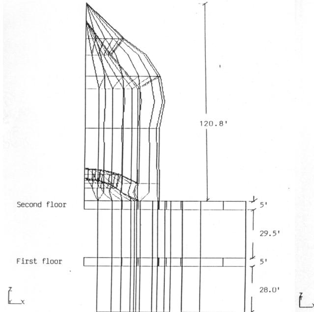
Figure 2 : Discretized view of dome super-element
