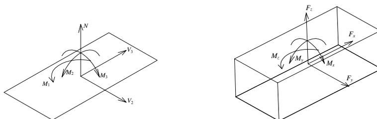
Figure 3 : Positive sign of interface stress resultants and external forces of single blocks
