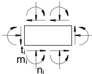
Figure 1 : Stress resultants applied to the single block
