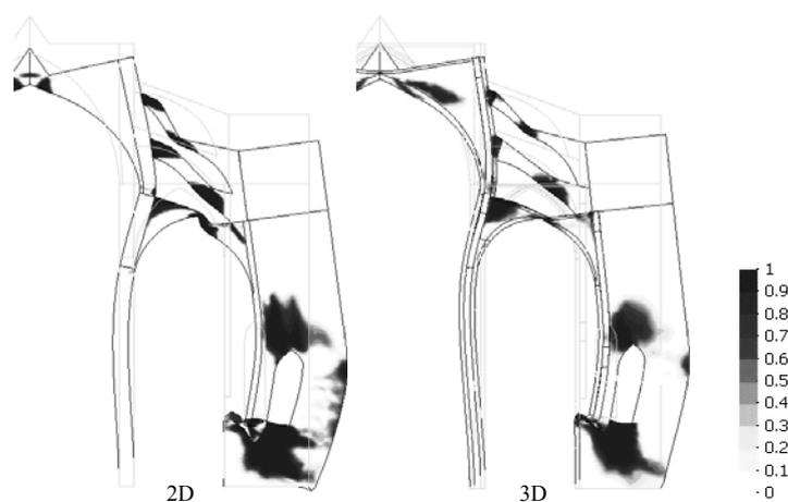
Figure 3 : Collapse mechanism and distribution of the tensile damage index under gravity loads with the smeared crack model
