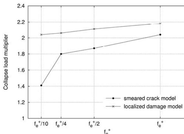
Figure 6 : Variation of the collapse gravity load multiplier in function of the tensile strength  $f_e^+$
