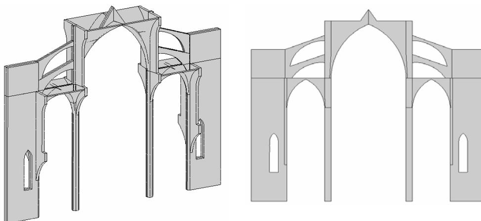
Figure 2 : 3D and 2D geometrical models of a typical bay
