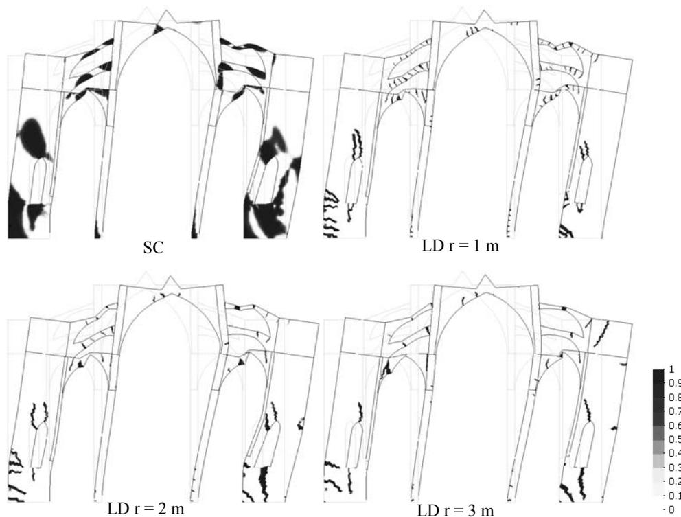
Figure 8 : Collapse mechanism and distribution of the tensile damage index under seismic loads for 2D models (SC: smeared crack model; LD: localized damage model; r: initial radius)
