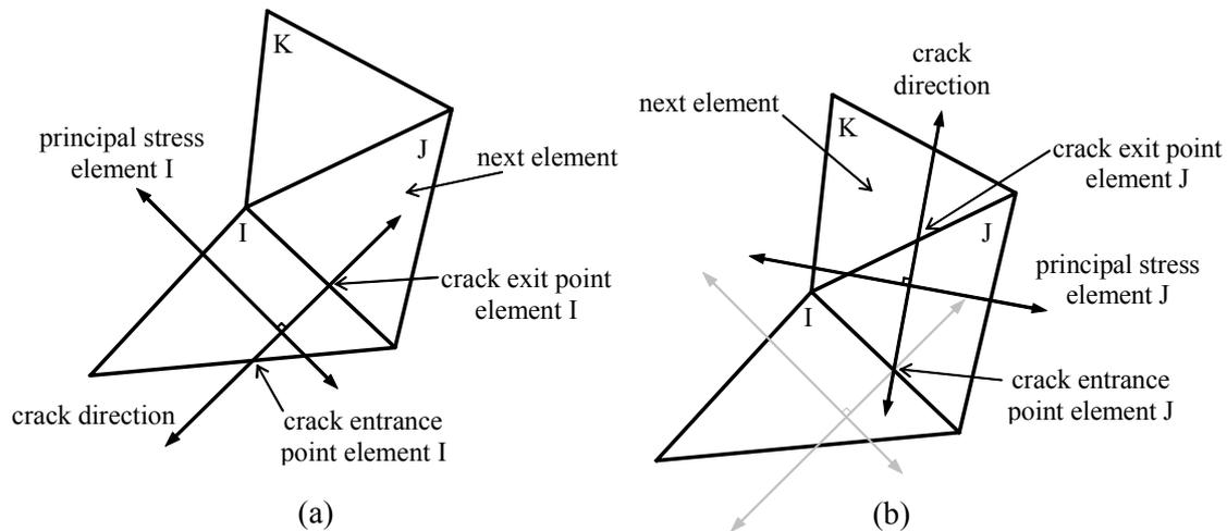
Figure 1 : (a) Exit point of element I (b) New potential element (J) and its entrance point
