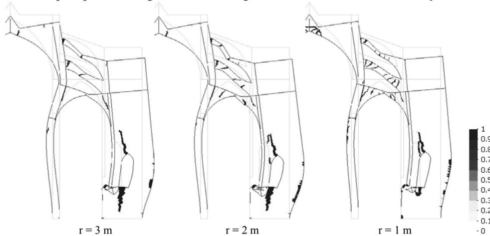
Figure 4 : Collapse mechanism and distribution of the tensile damage index under gravity loads with the localized damage model and different initial radius ( $r$ ) values
