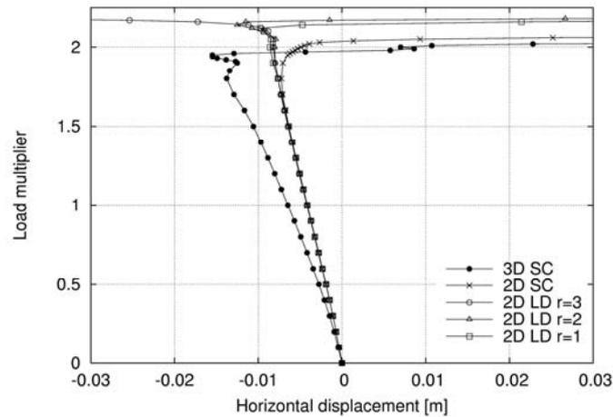
Figure 5 : Collapse load multiplier under gravity loads (SC: smeared crack model; LD: localized damage model;  $r$ : initial radius)
