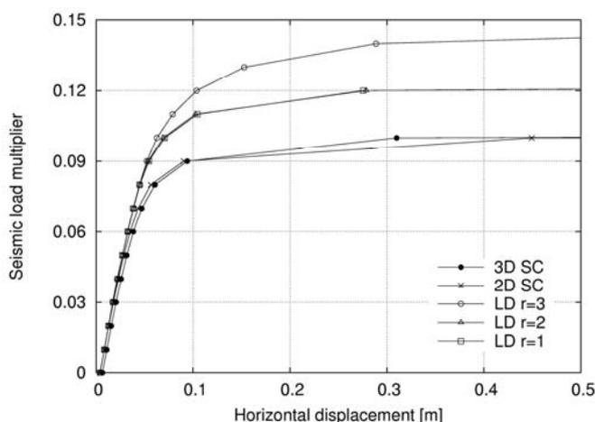
Figure 7 : Collapse load multiplier under seismic loads (SC: smeared crack model; LD: localized damage model; r: initial radius)
