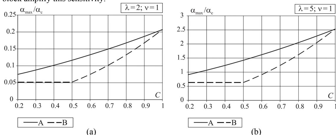
Figure 5 : Maximum angular displacement involved by the two schemes for different aspect ratios.
