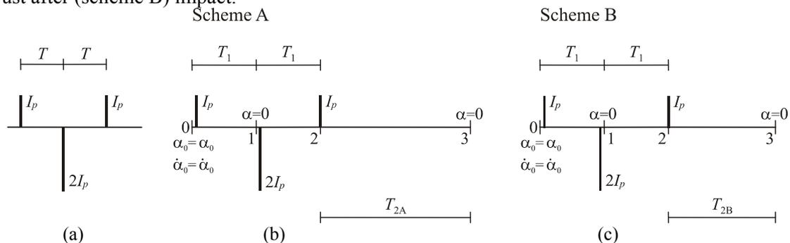
Figure 2 : (a) Assembly unit chosen to represent earthquake ground motion, with the second pulse acting: (b) just after impact (scheme A) and (c) just before impact (scheme B).
