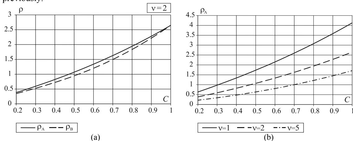
Figure 4 : Stability parameter versus  $C$ : (a) for both schemes A and B; (b) for scheme A only.
