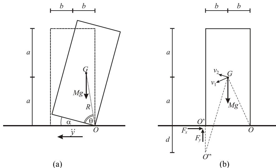
Figure 1 : (a) Rocking rigid block system; (b) velocities of the mass centre during impact.
