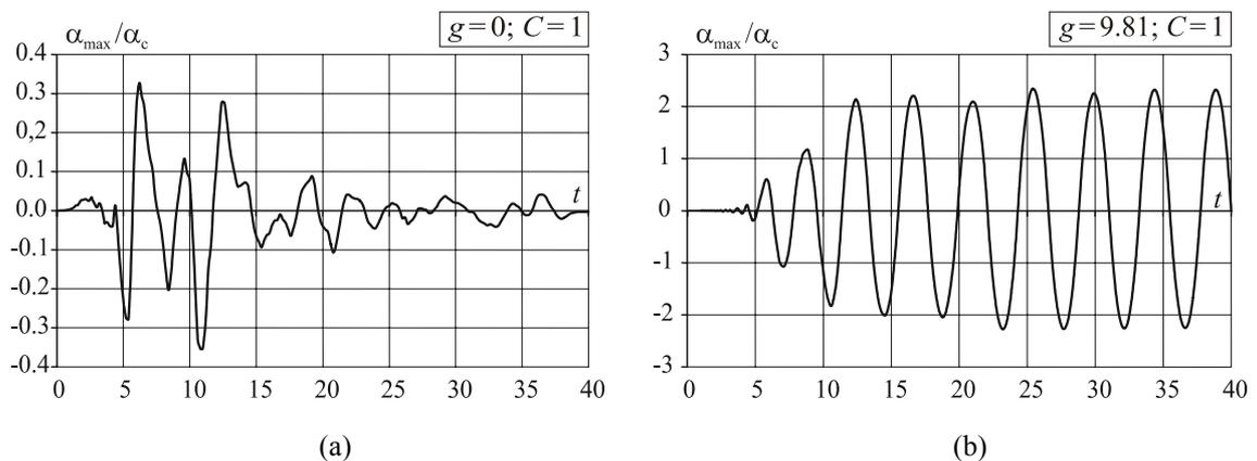
Figure 3 : Block response to the Sturno earthquake (Irpinia-Italy, 1980, PGA=0.25g): (a) gravity is neglected; (b) gravity is the cause of divergence.
