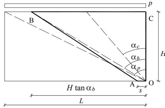
Figure 2 : Masonry wall with  $\alpha_b \leq \alpha_p$ . The solid line shows the equivalent area of wall considered for the calculation of the friction force.
