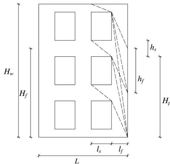
Figure 6 : Possible crack lines in a multistorey pier and spandrel. A uniformly distributed load due to the live loads and horizontal structures is assumed to act at each storey level.
