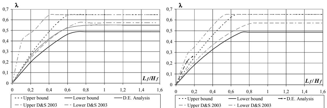
Figure 8 : Comparison for collapse load factor curves obtained with the discrete element analysis and two simplified approaches. Shape ratio  $s / h = 1.143$  and case a) one storey, b) two storeys.
