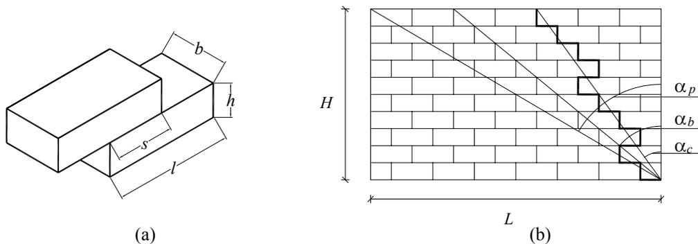
Figure 1: (a) Block dimensions; (b) inclinations for the unit and wall shape ratios and for the variable angle of crack.
