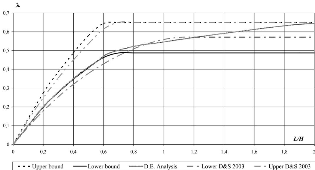
Figure 5 : Comparison for collapse load factor curves obtained with the discrete element analysis and two simplified approaches. Shape ratio  $s / h = 1.143$
