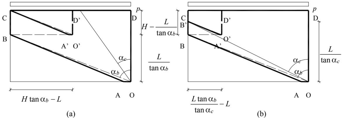
Figure 3 : Masonry wall with  $\alpha_b \geq \alpha_p$  and (a)  $\alpha_c \leq \alpha_p$  and (b)  $\alpha_c \geq \alpha_p$  Layout of the portions of wall considered for the calculation of the friction forces.
