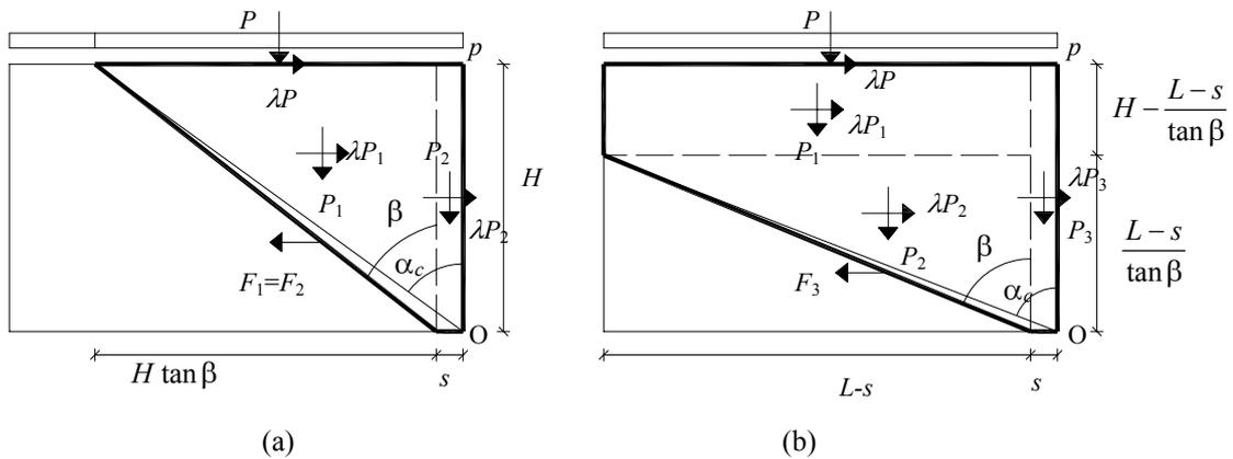
Figure 4 : Macro block identified by the angle of crack (a)  $\alpha_c \leq \alpha_p$  and (b)  $\alpha_c \geq \alpha_p$ .
