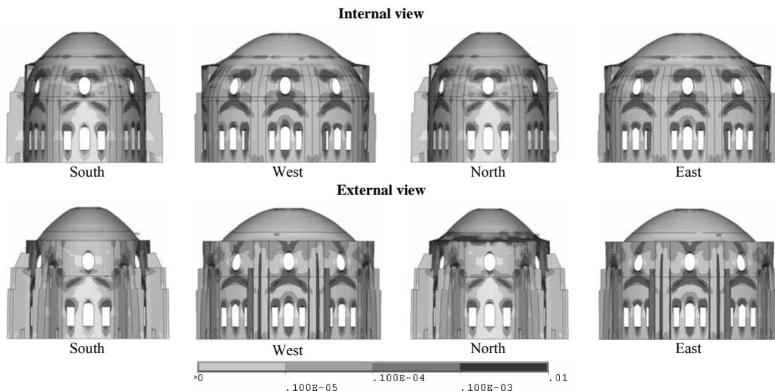
Figure 4 : Principal inelastic strains. Self-weight analysis.
