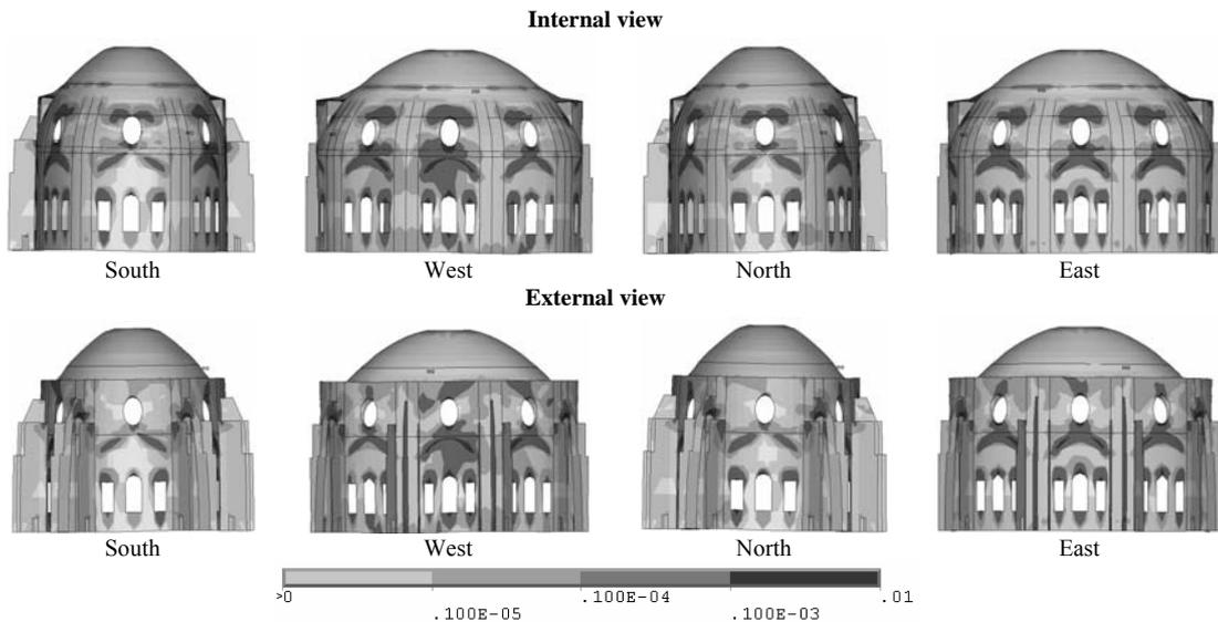
Figure 6: Principal inelastic strains. Settlement analysis.
