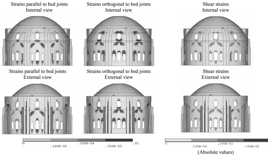
Figure 5: Inelastic strains in the local coordinate system of the elements (West side). Self-weight analysis.
