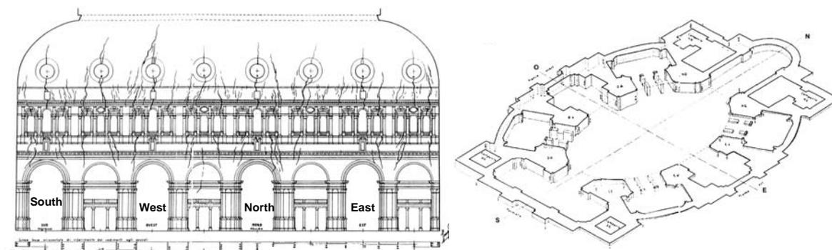
Figure 2 : (a) Crack pattern; (b) Axonometric view of total settlements.
