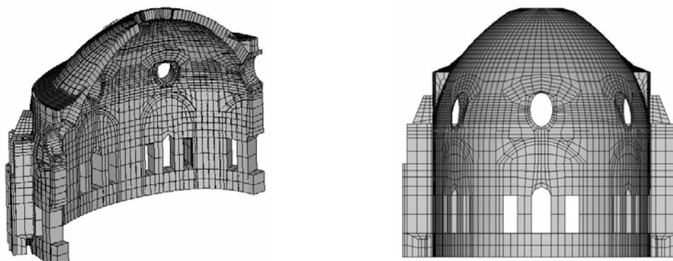
Figure 3 : FEM model of the dome-drum system.
