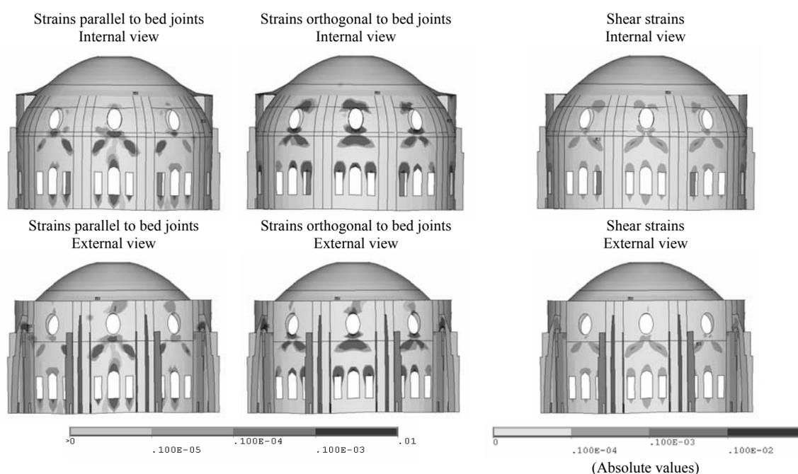
Figure 7: Inelastic strains in the local coordinate system of the elements (west side). Settlement analysis.
