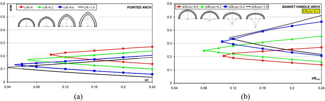
Figure 6 : Maximum and minimum thrust: (a) pointed arches; (b) basket handle arches.
