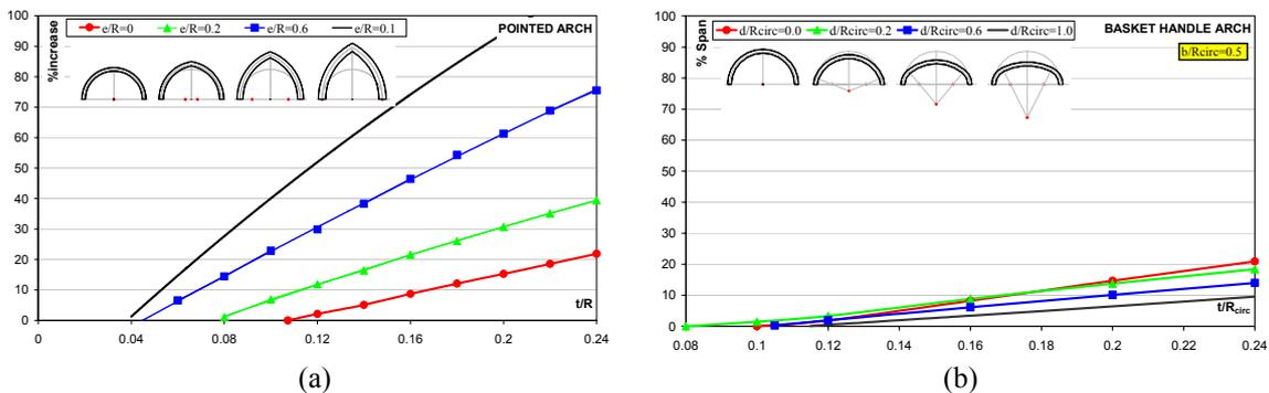
Figure 9 : Span increase in arches: (a) pointed arches; (b) basket handle arches.
