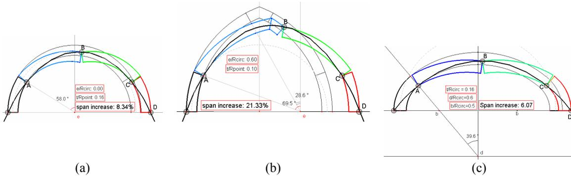
Figure 8 :Maximum displacements: (a) circular arch; (b) pointed arch; (c) basket handle arch.
