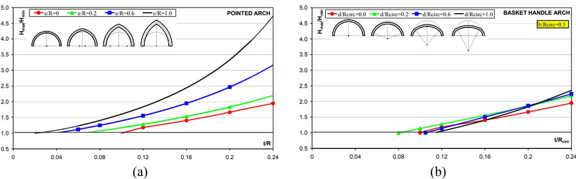
Figure 7 : Ratio of the maximum over the minimum thrust: (a) pointed arches; (b) basket handle arches.
