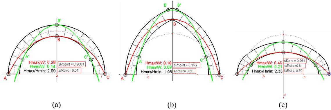
Figure 4 : Thrust lines: (a) circular arch; (b) pointed arch; (c) basket handle arch.
