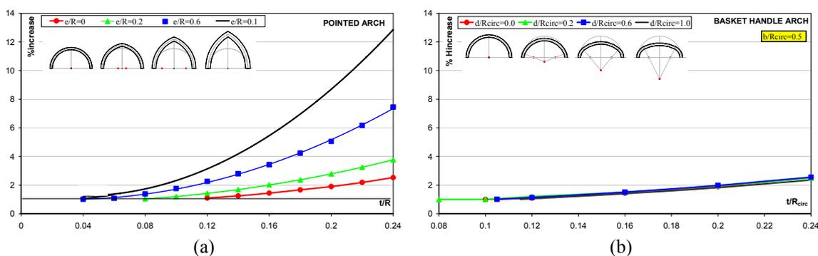
Figure 10 : Thrust increase due to the span increase: (a) pointed arches; (b) basket handle arches.
