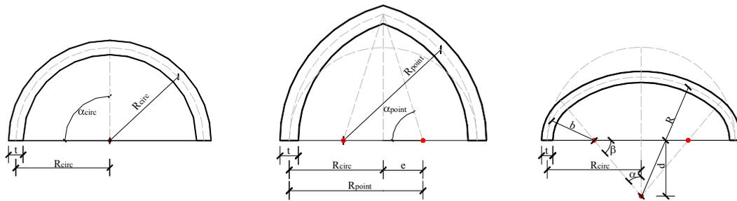
Figure 2 : Geometry definition for the three types of arches.
