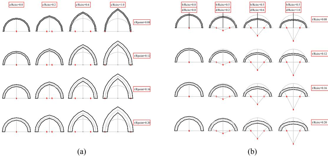
Figure 5 : Study cases varying the geometries: (a) pointed arches; (b) basket handle arches.
