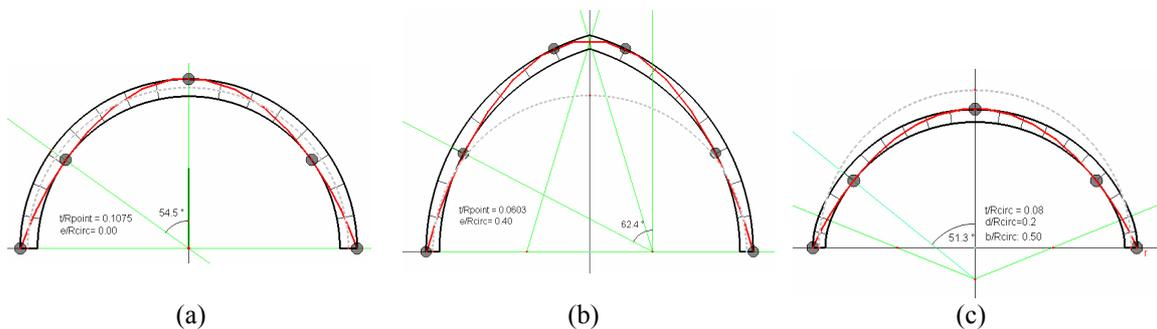
Figure 3 : Minimum thickness: (a) circular arch; (b) pointed arch; (c) basket handle arch.
