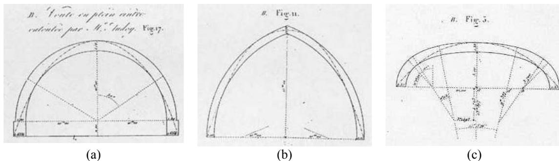
Figure 1 : Méry (1840) demonstrated thrust lines for arches of various shapes
