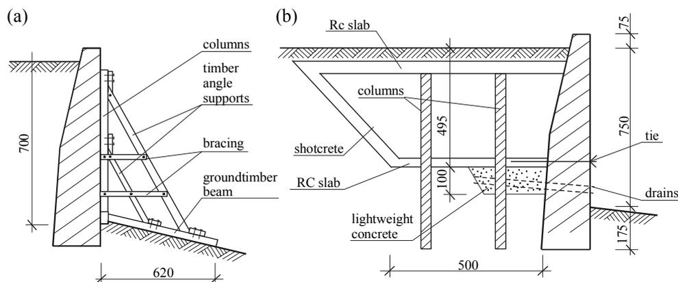
Figure 14 : Temporary supports of the retaining wall and the cross section through the unloading chamber.
