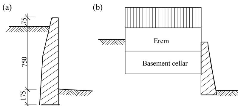
Figure 10 : The cross-section of the retaining wall with erems, (a) the retaining wall, (b) erems behind the wall.
