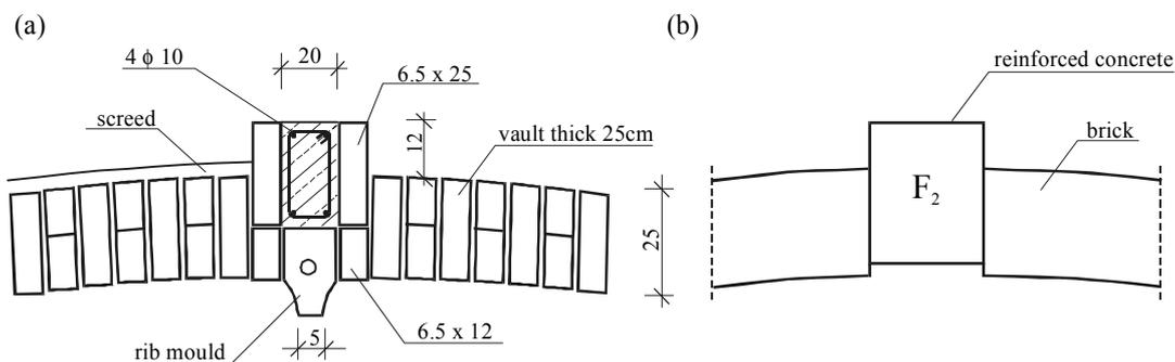
Figure 2 : The composite form of the reconstructed ribs of vault, (a) construction, (b) equivalent section.
