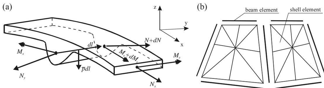
Figure 4 : Internal forces in the cross-section of a curved beam with shells.
