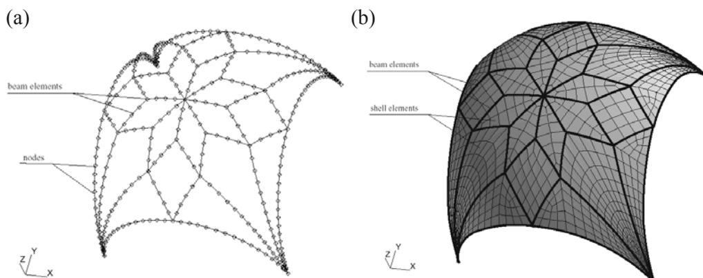
Figure 5 : Three-dimensional beam system of the structure and three-dimensional system of the arched beams with infilling shells.
