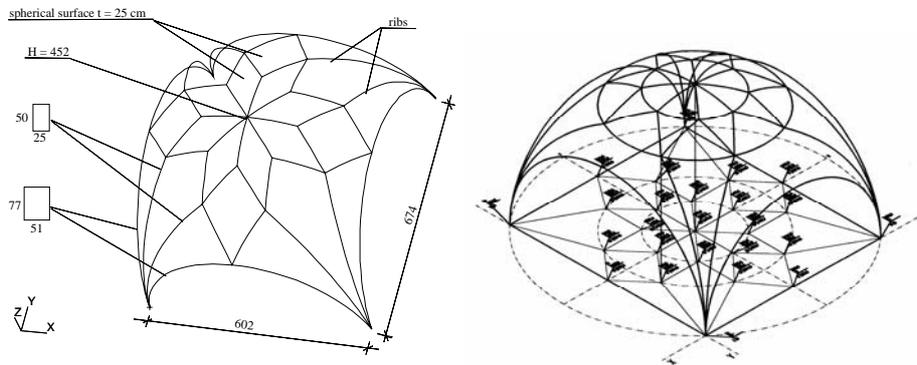
Figure 3 : Numerical modelling of the gothic stellar vault and its reproduced geometry.
