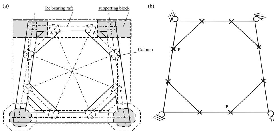
Figure 8 : The RC base-raft bearing the tower, (a) structure, (b) static diagram.
