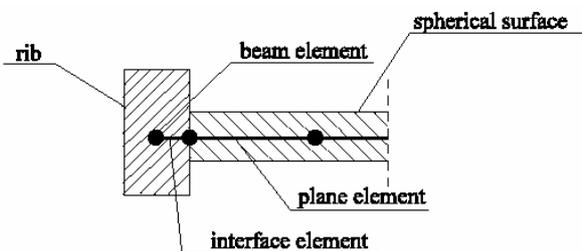
Figure 6 : Coupling of the beam and plane elements.
