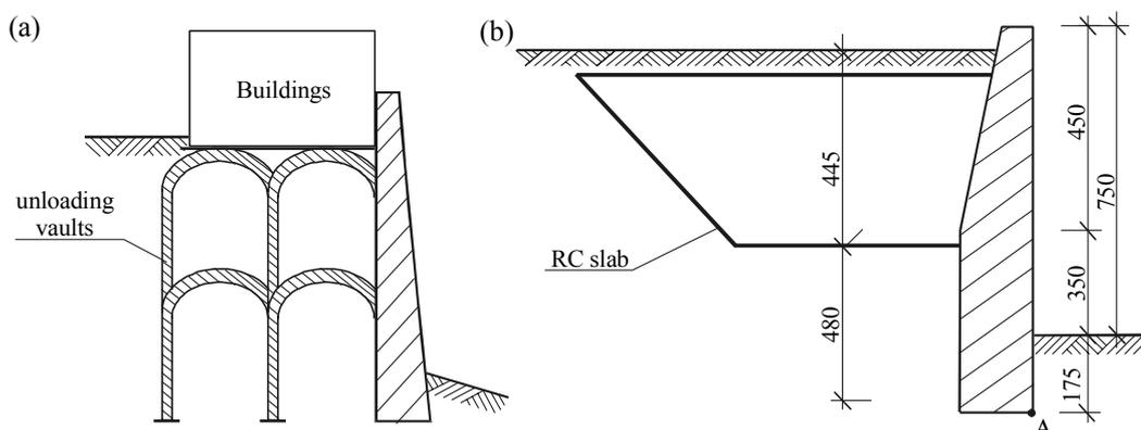
Figure 11 : Schemes of unloading vaults, (a) in the building cellars, (b) scheme of unloading chamber.
