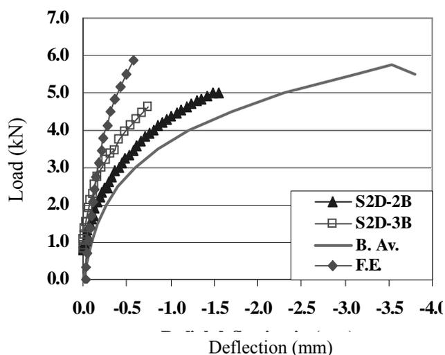
Figure 1 : Shallow arch load deflection curve
