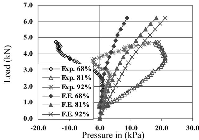
Figure 3 : Pressures at different location of deep arch
