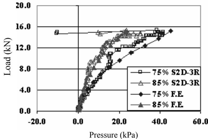
Figure 7 : Pressures at different sections of shallow repaired arch
