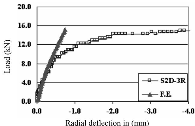
Figure 5 : Load arch deflection (Repaired shallow arch)
