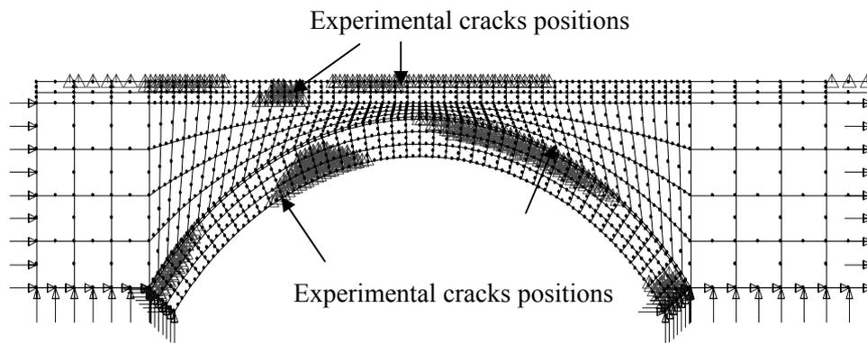
Figure 4 : Shallow repaired arch predicted hinge position
