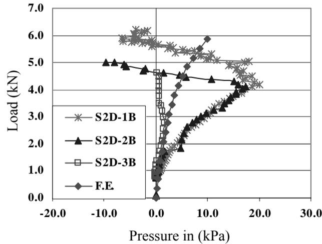
Figure 2 : Pressure on extrados of shallow arch (75 % span)
