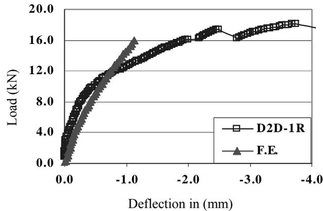
Figure 6 : Load arch deflection (repaired shallow arch)
