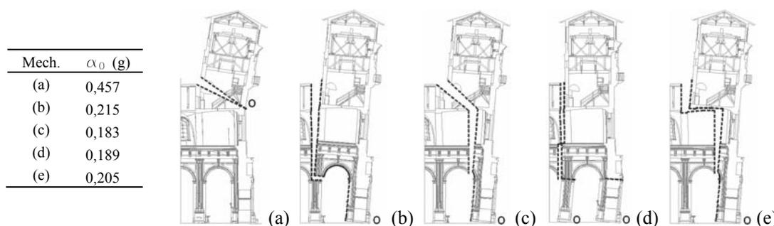
Figure 6 : (a) to (e): Considered façade out-of-plane overturning mechanisms, detail of the separation surfaces and hinge positioning, and obtained  $\alpha_0$  values.
