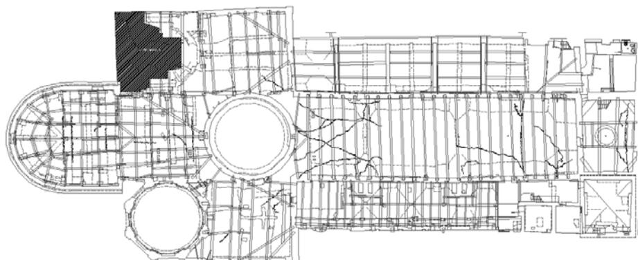
Figure 3 : View of the damage pattern reported on the vaults, mainly localized at the crossing between main nave and transept and in the façade area
