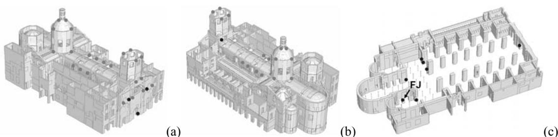
Figure 4 : Tests positioning, external view from North (a) South (b) and axonometric view, from East. Darker spots correspond to points of execution of direct sonic tests, lighter spots to dynamic identification sensors' positions.
