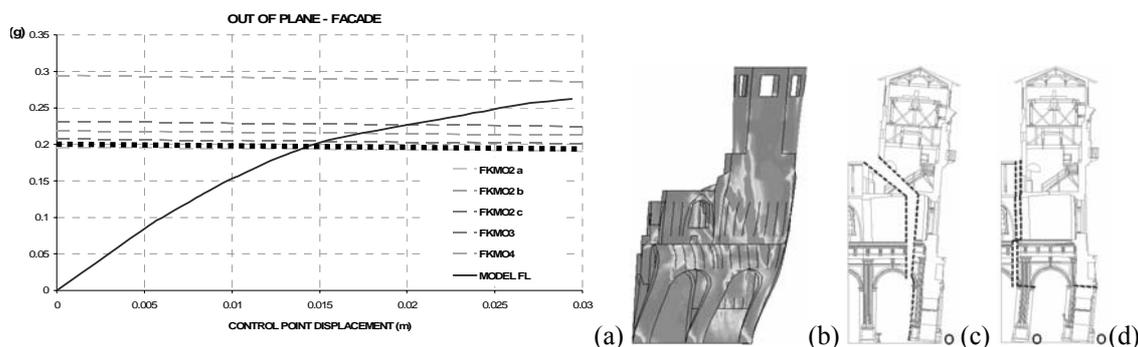
Figure 9 : Façade model, (a) FE and limit analysis capacity curves, the bold dotted black line corresponds to the almost coinciding kinematic models (c) and (d) capacity curves; (b) numerical outcomes at the last step of the non linear analysis (0.26 g); comparison with the limit analysis mechanisms (c) and (d).
