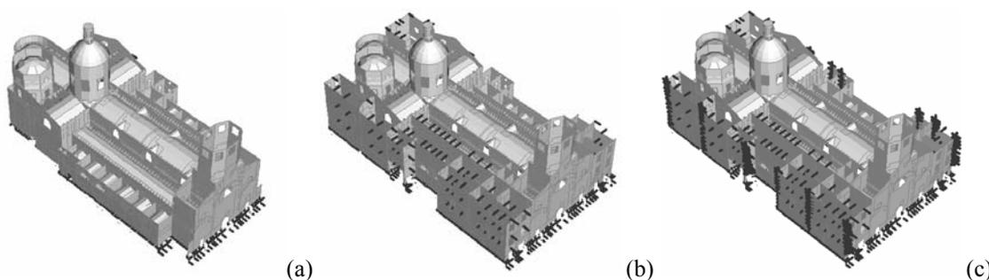
Figure 7 : From the first model (a) to the definitive (c) through successive boundary conditions variation.
