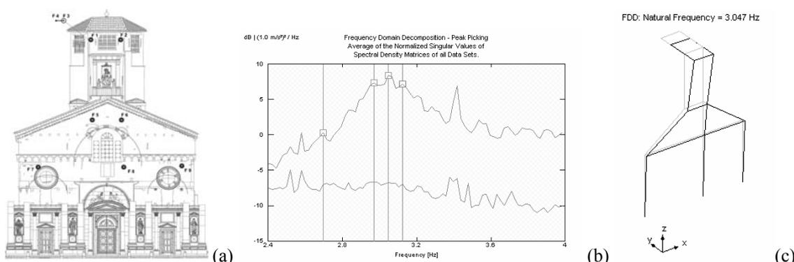
Figure 5 : Façade dynamic identification: (a) sensors positioning,; (b) Frequency Domain Decomposition Peak Picking method, selected frequencies; (c) defined mode shape, first (bending) resonant frequency
