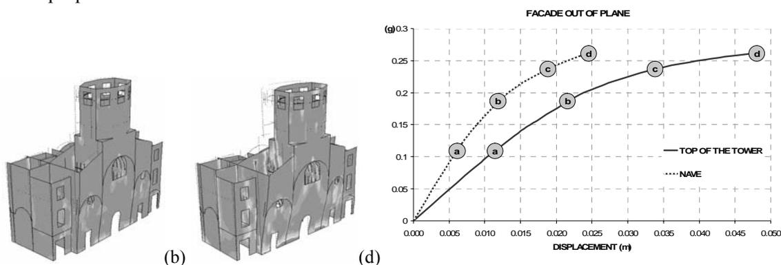
Figure 8 : Façade model, damage progression, maximum principal strains: the damage pattern denoted by the models in (b) -  $\alpha=0,19g$  - to (d) -  $\alpha=0,26g$  - is related to the corresponding points of the capacity curves (control points at the top of the tower and at the nave's level) in the diagram.
