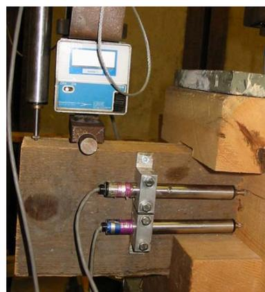
Figure 7 : Applied load jack.
