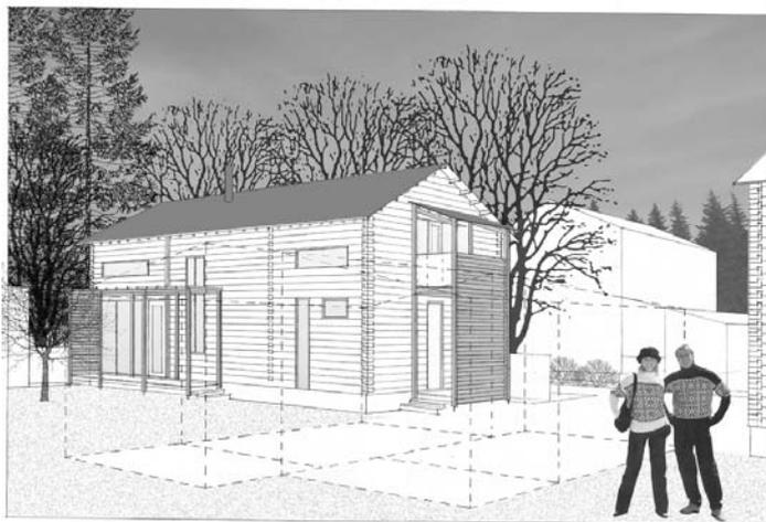
Figure 5 : A modern log house has a simple four-corner log frame like the traditional houses.
