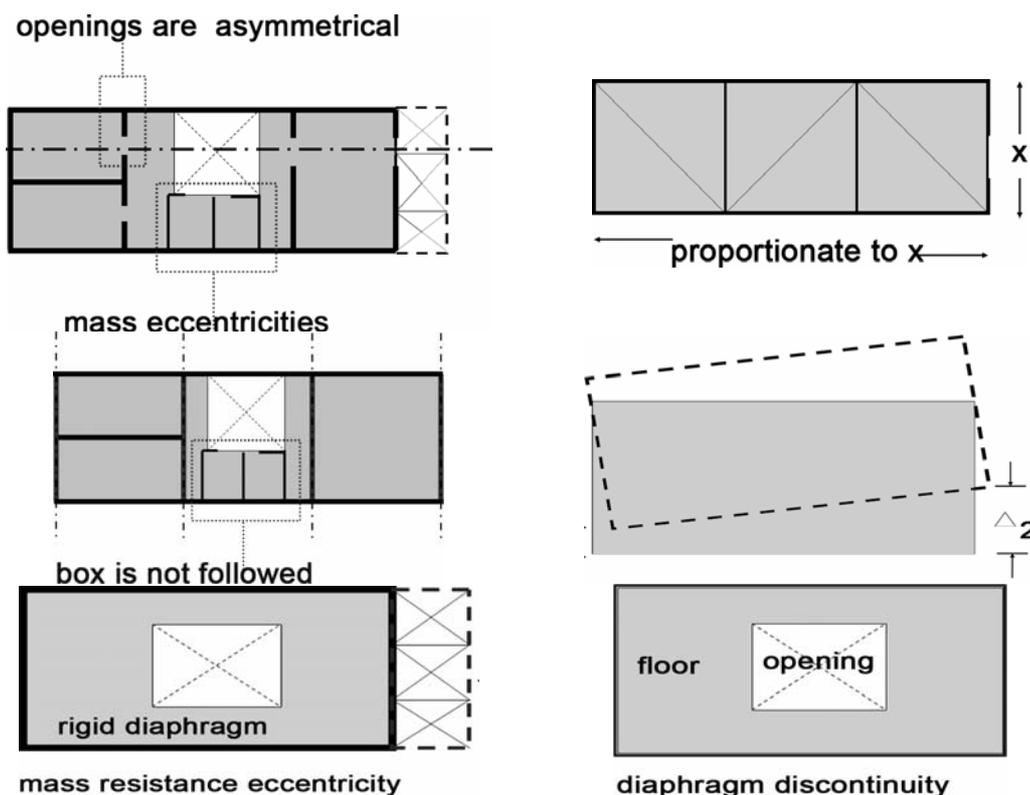
Figure 3 : Implications of the shape of the construction
