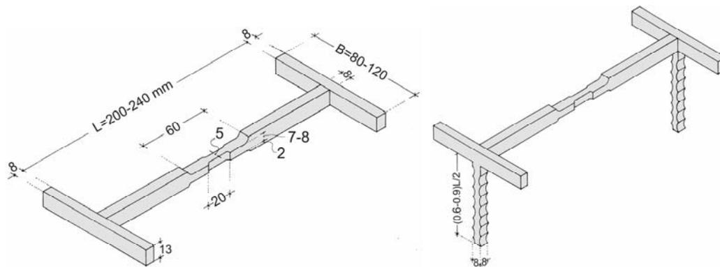
Figure 8 : The shape and the typical dimensions of the new titanium clamps, designed for the well preserved mortises (left) and for the damaged or severely deteriorated mortises (right).
