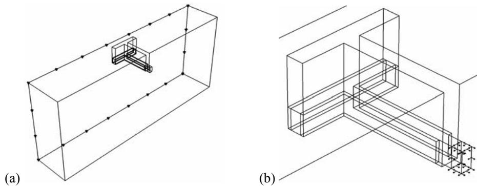
Figure 5 : Model with  $B = 8$  cm,  $L = 8$  cm and  $D = 5$  mm. (a) General view; (b) detail of the connection.
