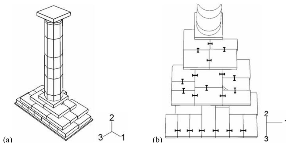
Figure 2 : Numerical model. (a) General view; and (b) location of the connecting elements (I).
