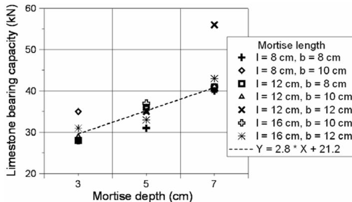
Figure 7 : The numerical results concerning the stone blocks bearing capacity in the area of the clamps.
