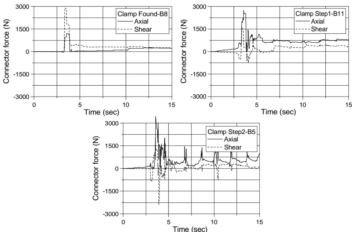
Figure 3 : The time histories of the connector forces that presented the greatest values at each stone layer
