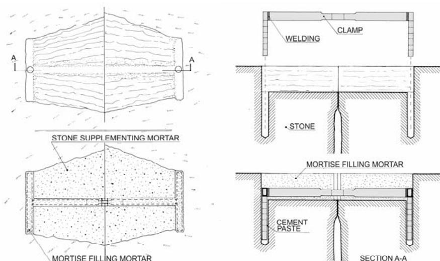
Figure 9 : Restoration of connections with damaged or severely deteriorated mortises.
