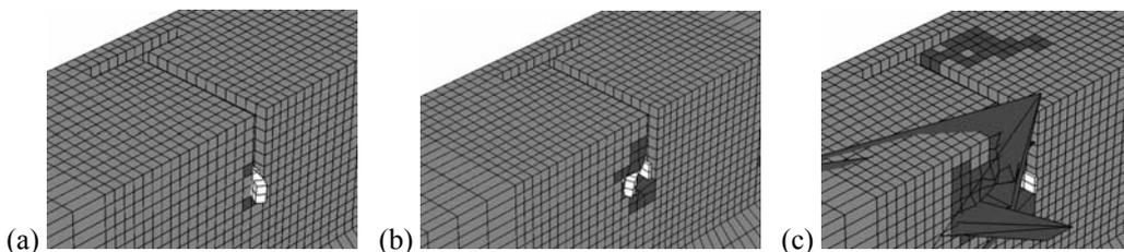
Figure 6 : Failure process of model with  $b = 10$  cm,  $l = 12$  cm and  $d = 7$  mm: (a) shear cracking initiation; (b) crushing of the mortise vertical edge; and (c) tensile cracking and half mortise destruction.
