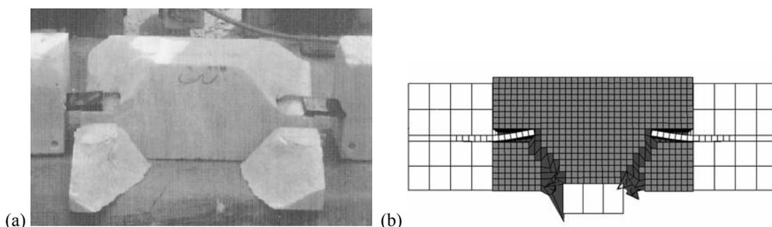
Figure 4 : (a) Fractured marble after the experiment (Zampas 1994). (b) Deformed model at the instance of total failure. The darker grey shade indicates the cracked elements that were removed from the mesh.
