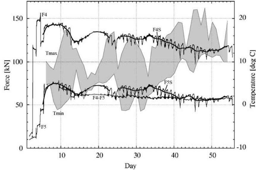
Figure 5: Forces in the tie-rods of section 4 ( $F4$ ) and section 5 ( $F5$ ); smoothed signals:  $F4S$ ,  $F5S$ ; exterior temperatures: daily minimum:  $Tmin$ , daily maximum:  $Tmax$
