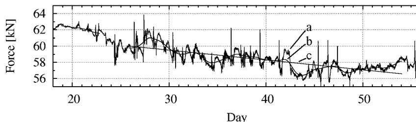
Figure 8: a:  $F_4-F_5$ : differences between forces in the Western and Eastern tie-rods, b: smoothed signal, c: linear regression
