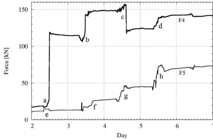
Figure 4 : Forces in the tie-rods during the dismantling of the flying buttresses
