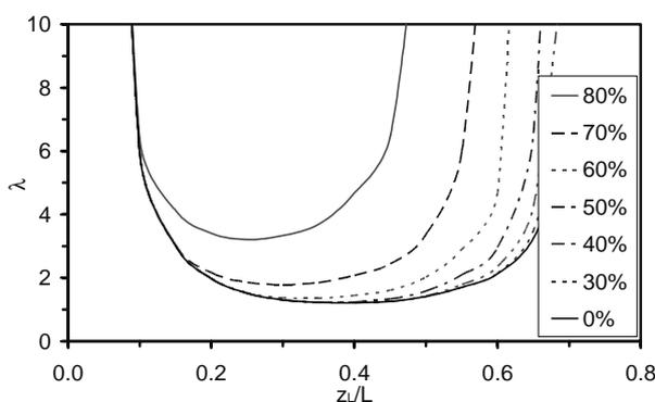
Figure 5 : Increase in load bearing capacity versus  $z_L/L$  for different ratios  $s_{FRP}/s_{ARCH}$  in the case of FRP at the intrados
