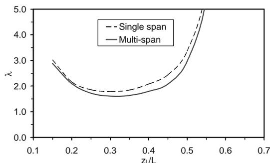
Figure 9 : Load factor  $\lambda$  versus  $z_L/L$  for single span and multi-span arch bridges.
