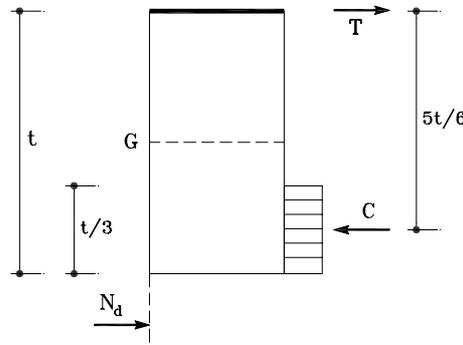
Figure 3 : Equilibrium of the reinforced cross-section
