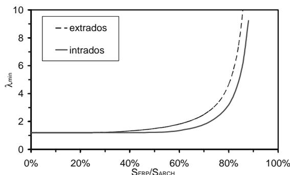
Figure 6 : Minimum load factor against  $s_{FRP}/s_{ARCH}$
