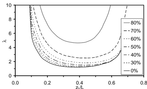
Figure 4 : Increase in load bearing capacity versus  $z_L/L$  for different ratios  $s_{FRP}/s_{ARCH}$  in the case of FRP at the extrados.
