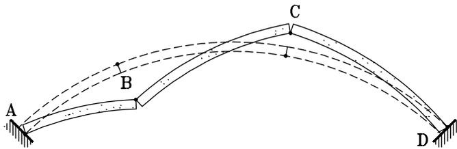
Figure 1 : Collapse mechanism of a masonry arch
