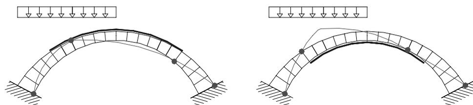
Figure 4 : Hinge locations and thrust line for FRP at the extrados and at the intrados
