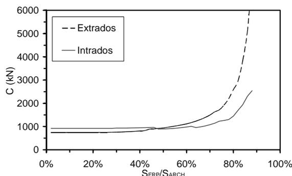
Figure 7 : Compression force against the values of FRP length
