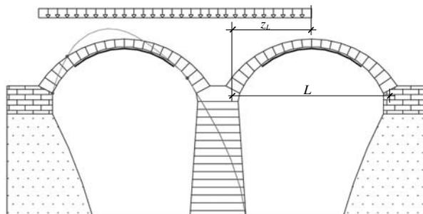
Figure 8 : The collapse of the pier
