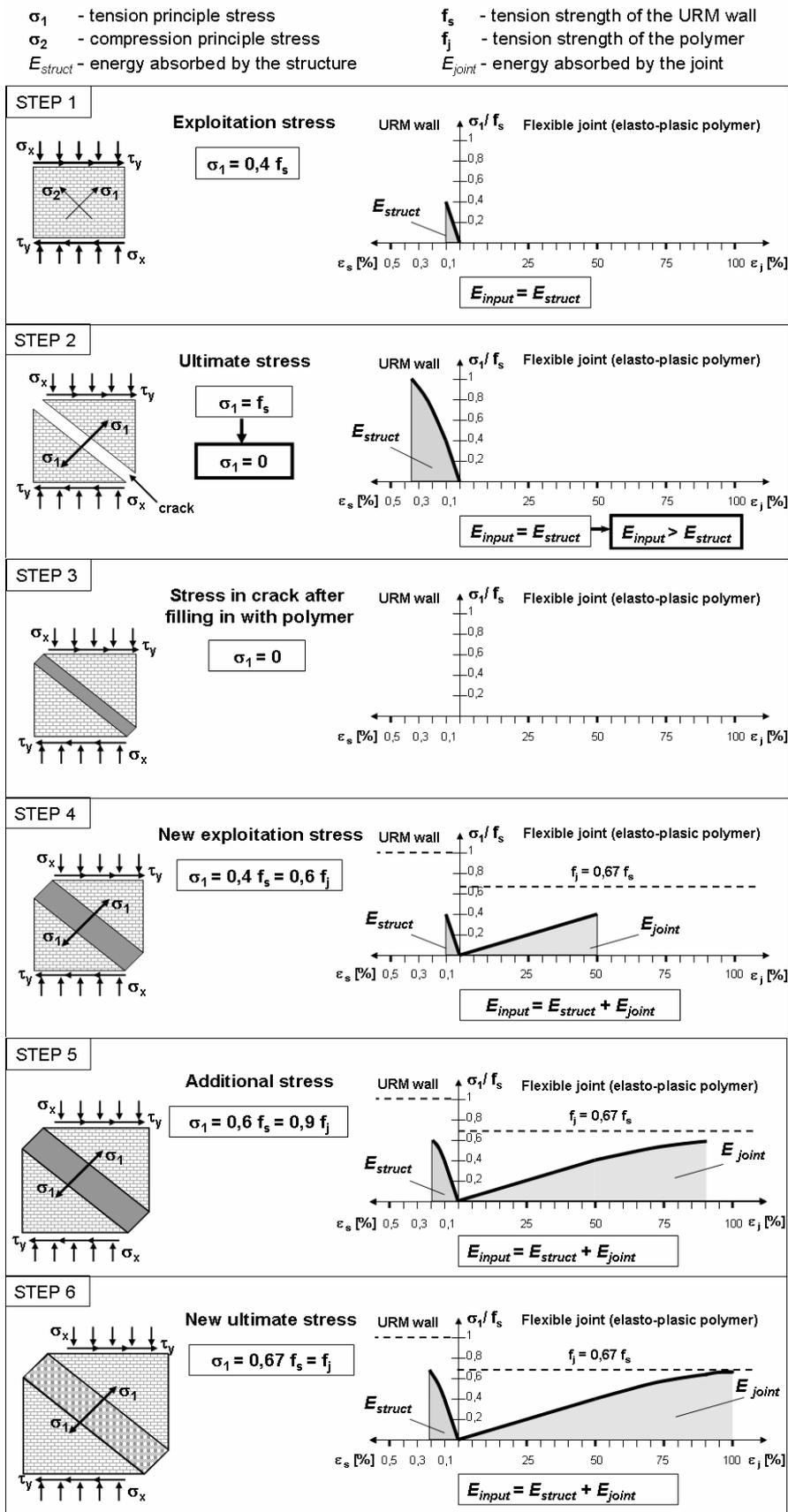
Figure 2 : Diagrams describing cooperation of a flexible joint with a cracked structure after application, working together under an additional load (based on the energy approach)
