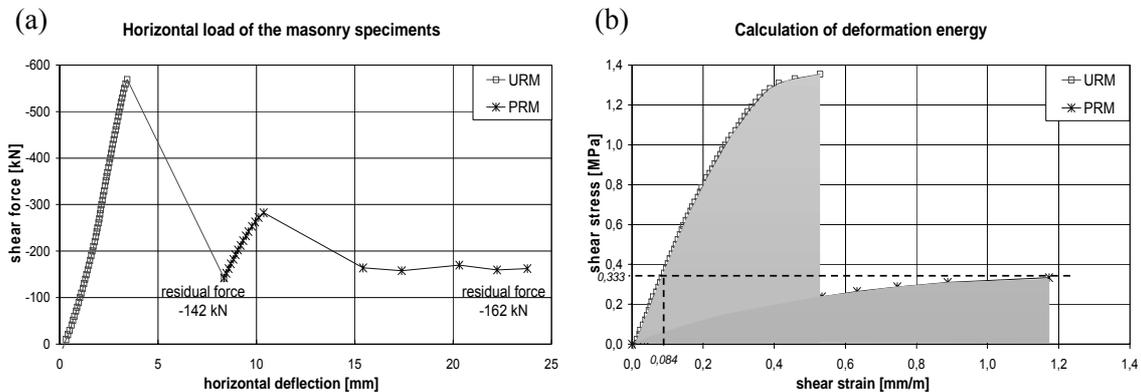
Figure 5 : Comparison of the URM and the PRM specimens: (a) History of loading and observed deflection; (b) Average stress-strain curves with calculation of deformation energy;
