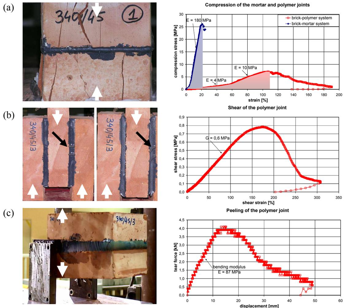
Figure 4 : Tests of brick specimens: (a) Compression of the 340/45 joint and mortar joint with comparison of deformation energy; (b) Shearing of the 340/45 joint; (c) Peeling of the 340/45 joint;
