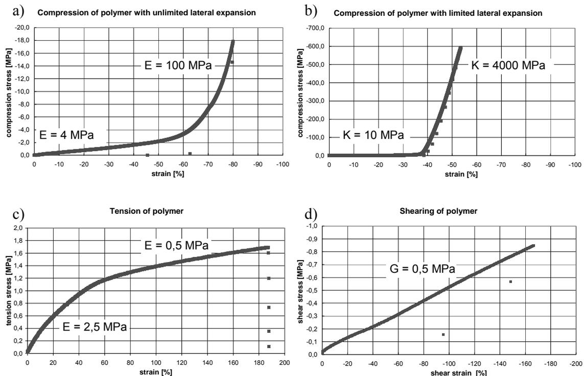
Figure 3 : Results of strength tests of polyurethane polymer 340/45: (a) Unlimited compression test with given Young's modulus  $E$ ; (b) Limited compression test with given bulk modulus  $K$ ; (c) Tension test with given Young's modulus  $E$ ; (d) Shear test with given shear modulus  $G$
