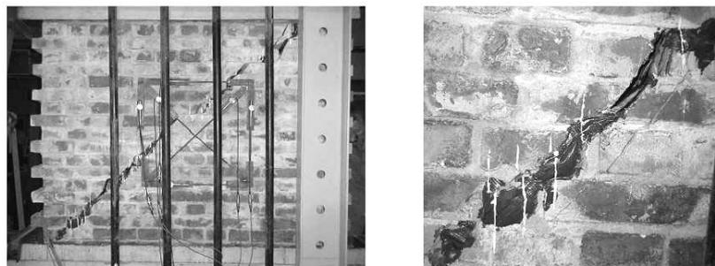
Figure 6 : The PRM specimen just after lost of the joint strength and focus on deformation of the joint
